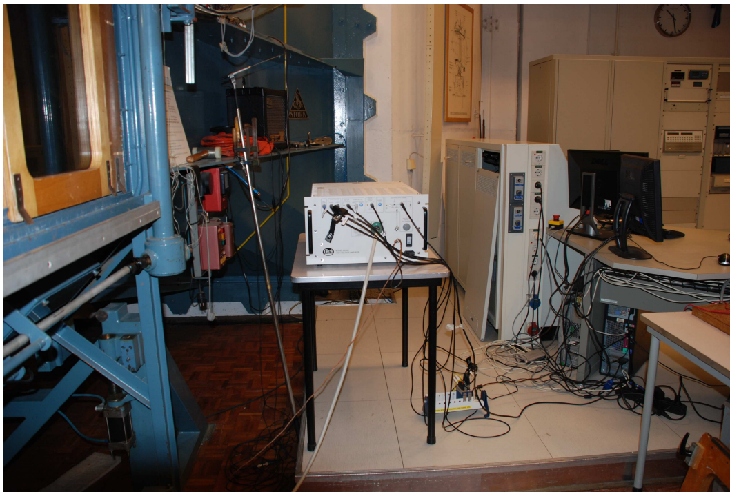
Figure 5.12: The TREK 20/20C HV amplifier placement in the LTT.
