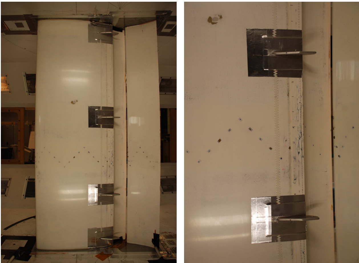
Figure A.2: Four metal support elements were attached to the lower surface of the airfoil, left from previous research. The elements were used to attach a cylindrical rod for vortex shedding. Because of possible follow-up studies with this configuration, it was decided to leave those elements attached.
