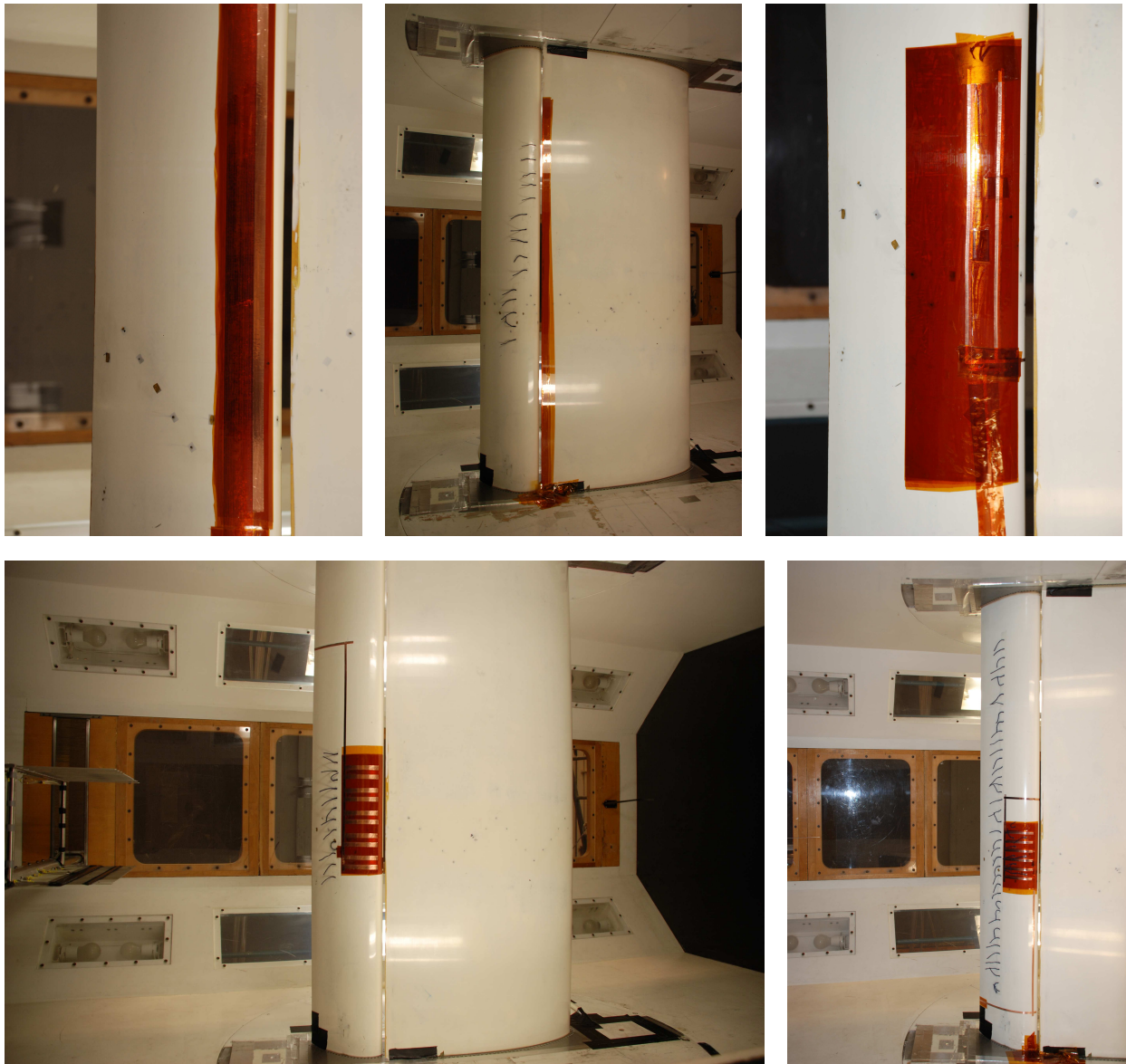
Figure A.3: Different plasma actuator configurations. From left to right and top to bottom: AC DBD plasma actuator, NS DBD plasma actuator, two parallel NS DBD plasma actuator, DBD-VG for counter-rotating vortices and DBD-VG for co-rotating vortices.
