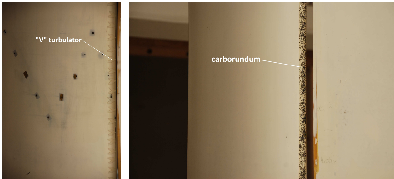
Figure 5.5: “V” turbulator (l) and carborundum 30 grains (r) on flap’s LE.
