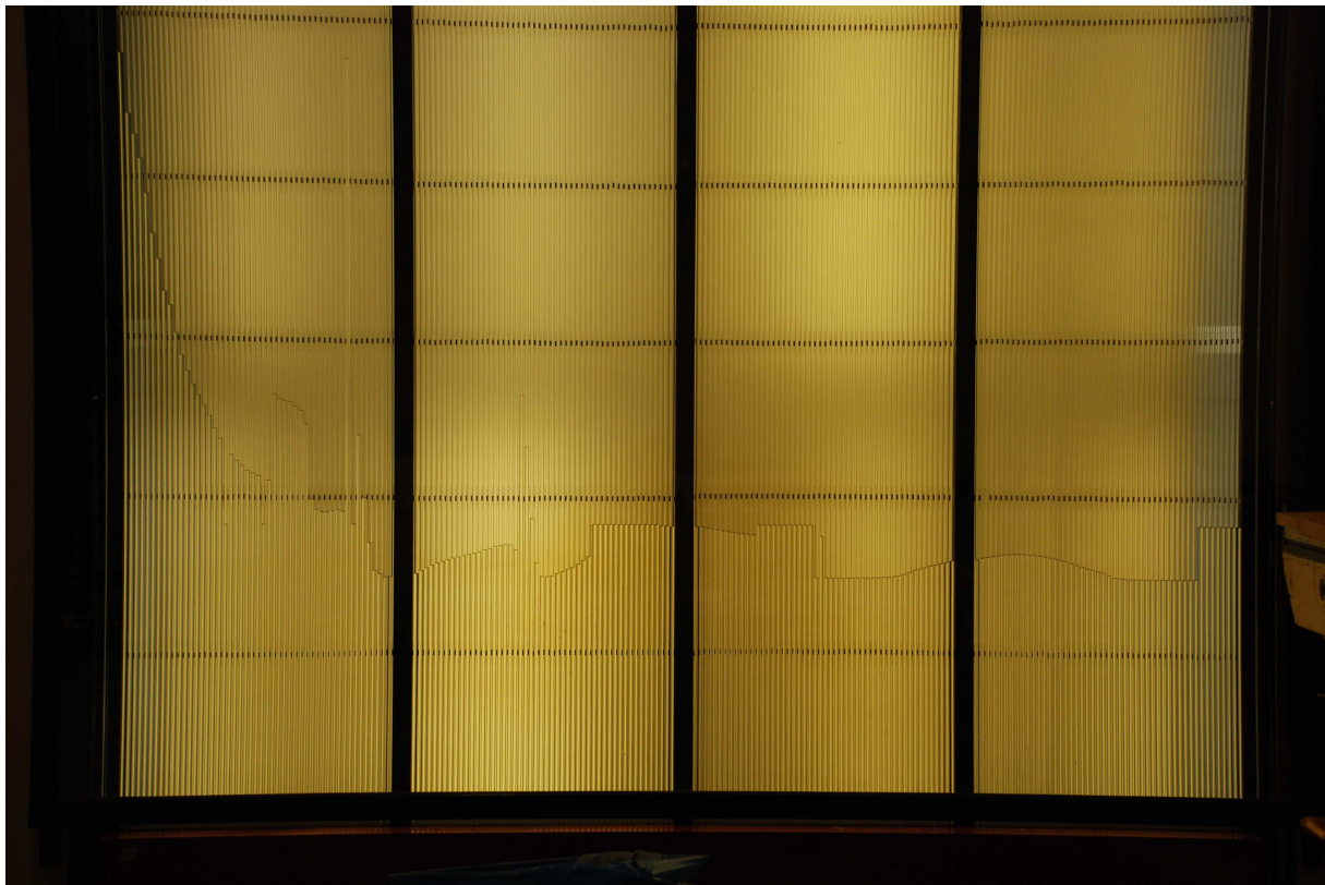
Figure 4.10: The multi-manometer for pressure monitoring.
