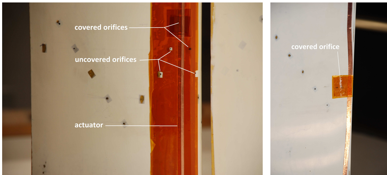
Figure 5.11: Some precautions for the actuator. Left: a dark rectangular area were multiple layers of dielectric are placed to prevent discharge with the metal orifice. Also some orifices could be uncovered to acquire more data. Right: prevention of discharge at the flap lower side where the high voltage connection was led.
