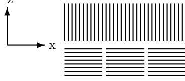
Figure D.1: Director profile in the bulk region of an uniaxially anisotropic medium with a surface of discontinuity at z = 0 . If z < 0 , \hat{\mathbf{d}} = (1, 0, 0) , and if z \geq 0 , \hat{\mathbf{d}} = (0, 0, 1) . The refractive indices n_o and n_e are independent of position.
