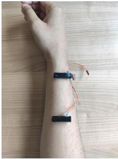
Fig 3. The vibrotactile actuators placed on the forearm and hand using double sided tape.
