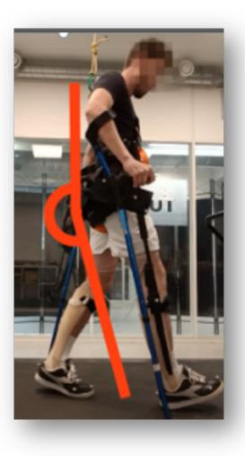
**Figure 2-2:** Extending the upper body will put tension in the upper spring at the back of the Cloud Walker. When lifting a leg the tension in the spring will swing the leg forward.
