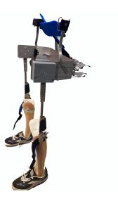
**Figure 2-1:** The complete side view of the final first prototype of the Cloud Walker. The leg parts and waist fixation are from an ARGO. The hip frame is self designed.
