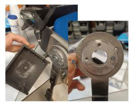
(a) Left hip; Dam- (b) Left joint; loose age in the cap caused screws and smoothed by the cable and cable edges caused by cable clamps. friction.
