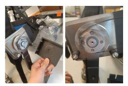
(c) Right hip; Dam- (d) Right age in the cap caused joint;Smoothed by the cable and cable edges caused by cable clamps. friction.
