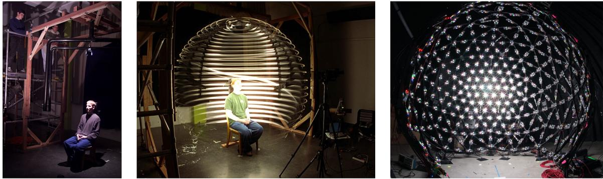
Figure 3.1: Left and center: Light stage gantry and acquisition timelapse of the Light Stage used by Debevec et al. [10]. Right: Light Stage used by Meka et al. [34].
