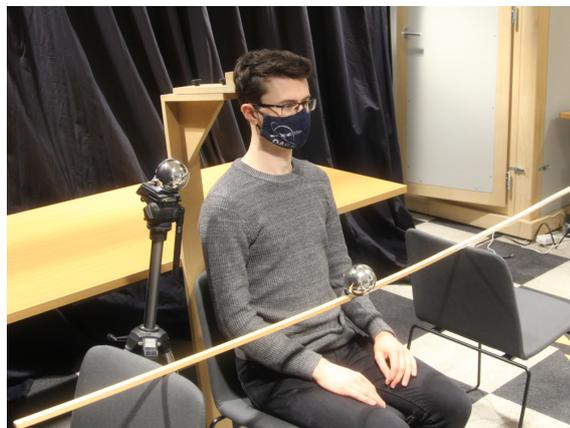
Figure 4.5: Left: Schematic acquisition setup. A camera captures the subject's face a flashing light source is manually moved around the subject. A simple reflective sphere is placed near the subject to retrieve the light direction from the images. Right: Studio acquisition setup. We placed two reflecting spheres for testing purposes, but we only require one.
