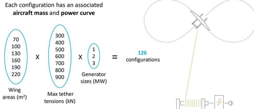
Figure 4.2: Design space input for case study
