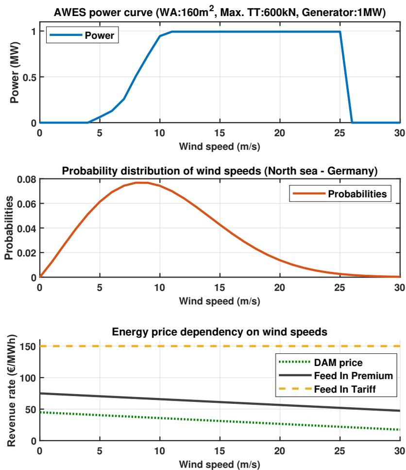
Figure 3.17: Revenue modelling based on energy price as a function of wind speeds
