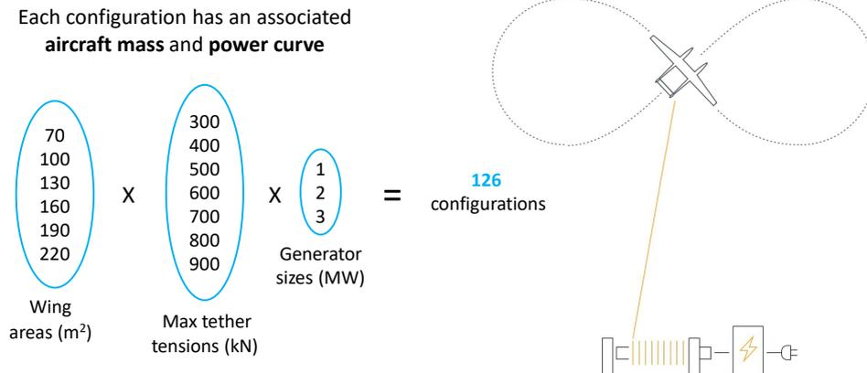
Figure 3.2: Sample design space generated from Ampyx Power's analytical performance model
