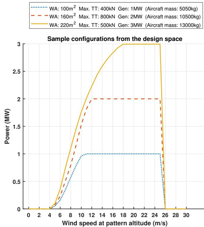
Figure 3.3: Sample AWES configurations from the generated design space
