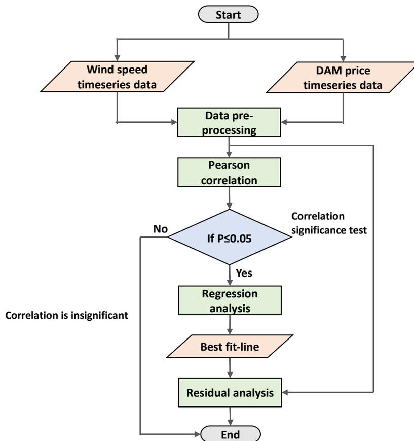
Figure 3.4: Flowchart of the correlation modelling method of DAM price and wind speeds
