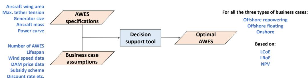
Figure 3.1: Framework of the developed decision support tool
