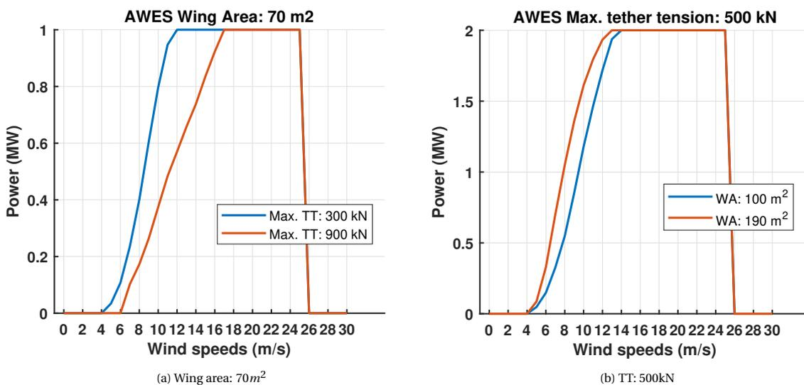
Figure 4.12: Sample power curves from design space showing different power production profiles at low wind speeds
