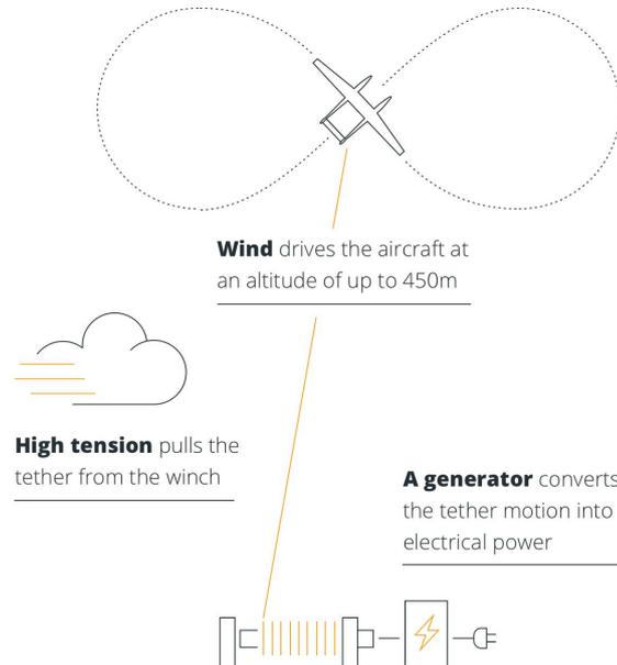
Figure 1.4: Technology schematic of Ampyx Power technology (Rigid wing aircraft with crosswind flight operation and ground based electricity generation) [5]
