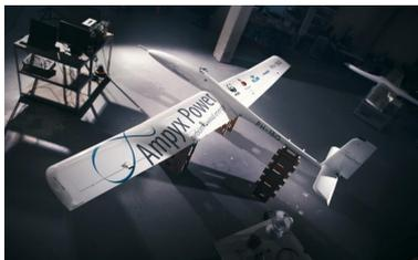
**AP-2** is used as an algorithm test bed
