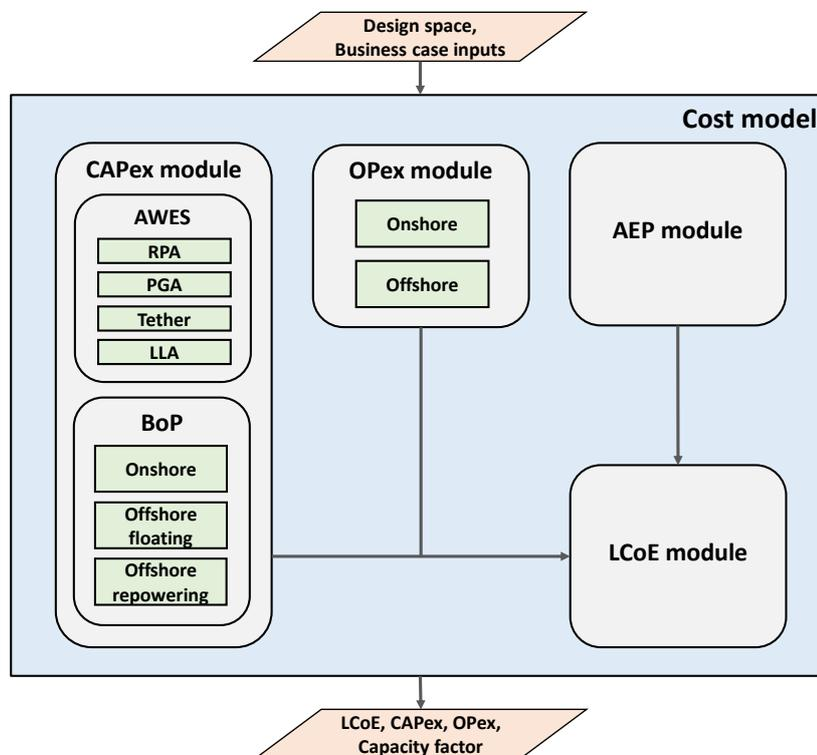
Figure 2.6: Current cost model of Ampyx Power AWES
