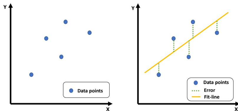
Figure 3.11: Representation of Ordinary Least Squares method for linear regression analysis
