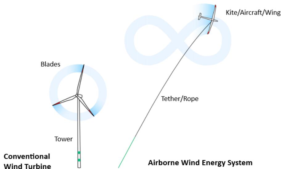
Figure 1.1: Analogy of AWES with conventional wind turbines [2]
