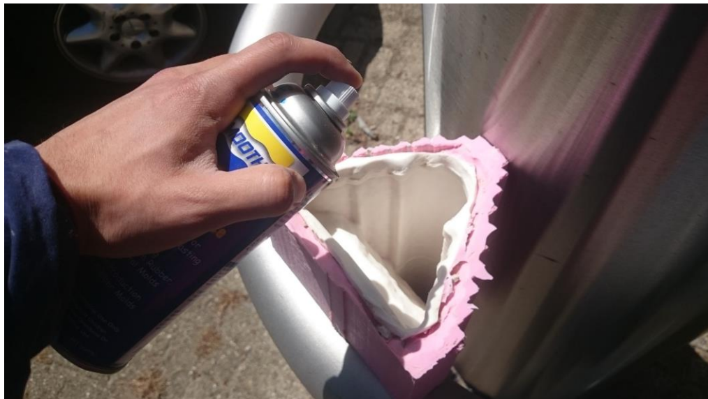
Release agent applied to inside
