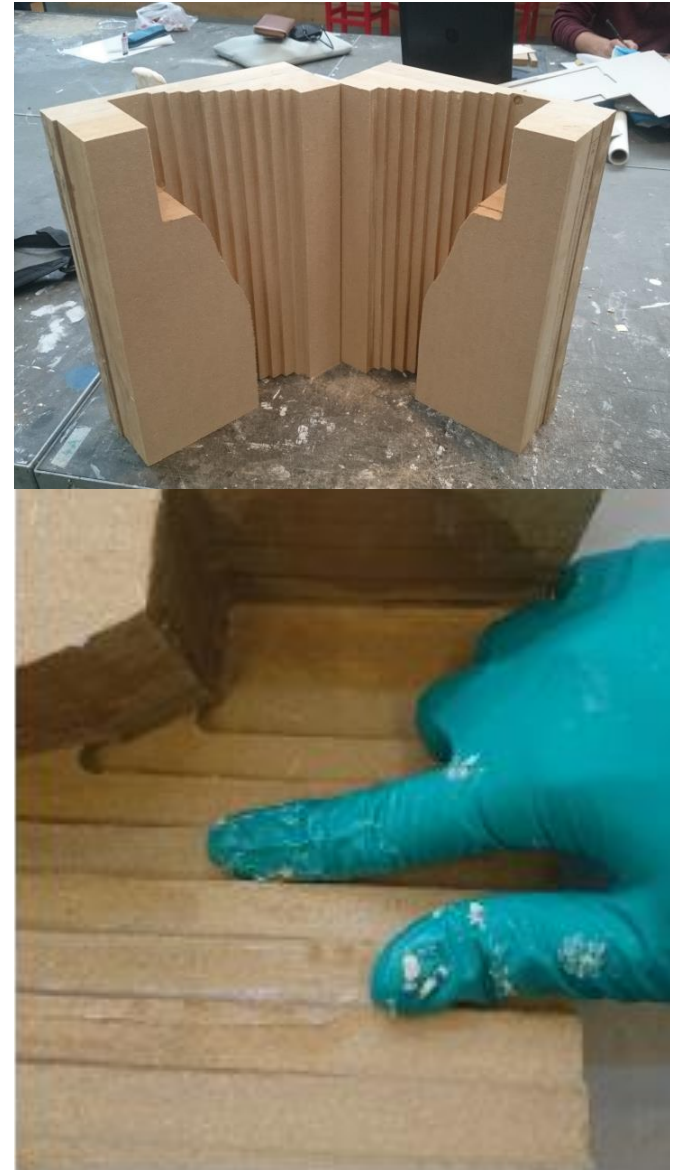
Release agent applied to the MDF mold reinforcement
