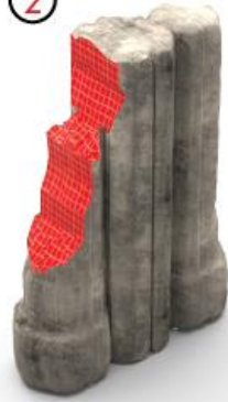
Surface replication of fracture morphology (LIDAR)
