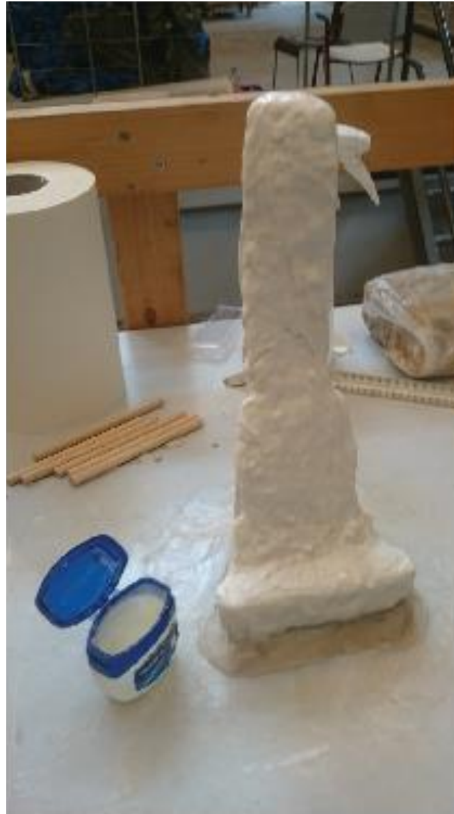
Held down with clay and release agent applied (clay only)
