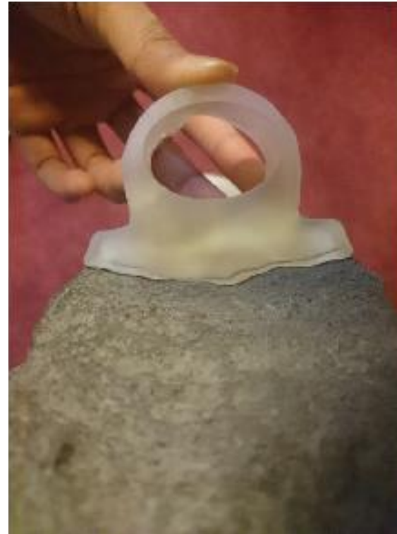
SLA Printing (Form 1+) failed prints
