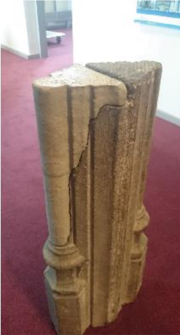
First cast (no aggregate and 10 g white pigment)
