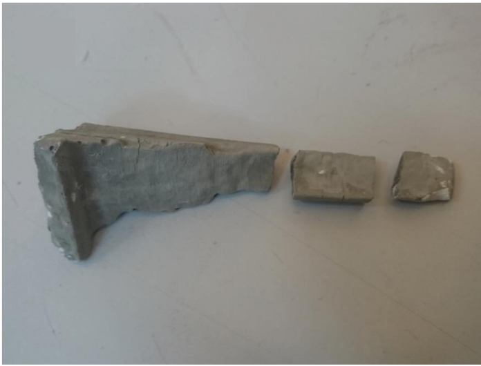
Bubbles would cause regular breakage.
