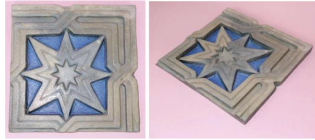
Pro-Jet - Powder Infiltrate (Most expensive but colored and accurate)
