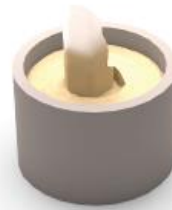
Polymer 'pattern' is dipped in Silica slurry or alternatively stuccoed
