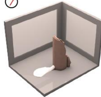
The oven is first heated to around 200°C (for Nylon 6) to remove the polymer 'pattern' and then at 900°C for sintering.
