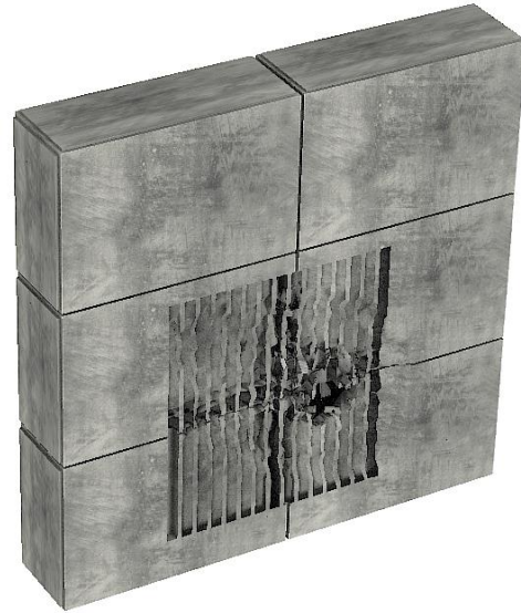
Step 2 Relief cuts for removal
