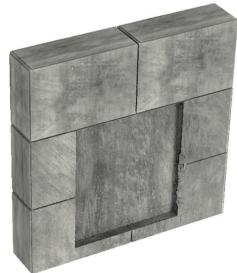
Step 3 Material chiseled out
