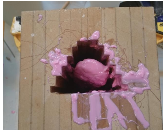
Silicone was poured with 2 cm margin
