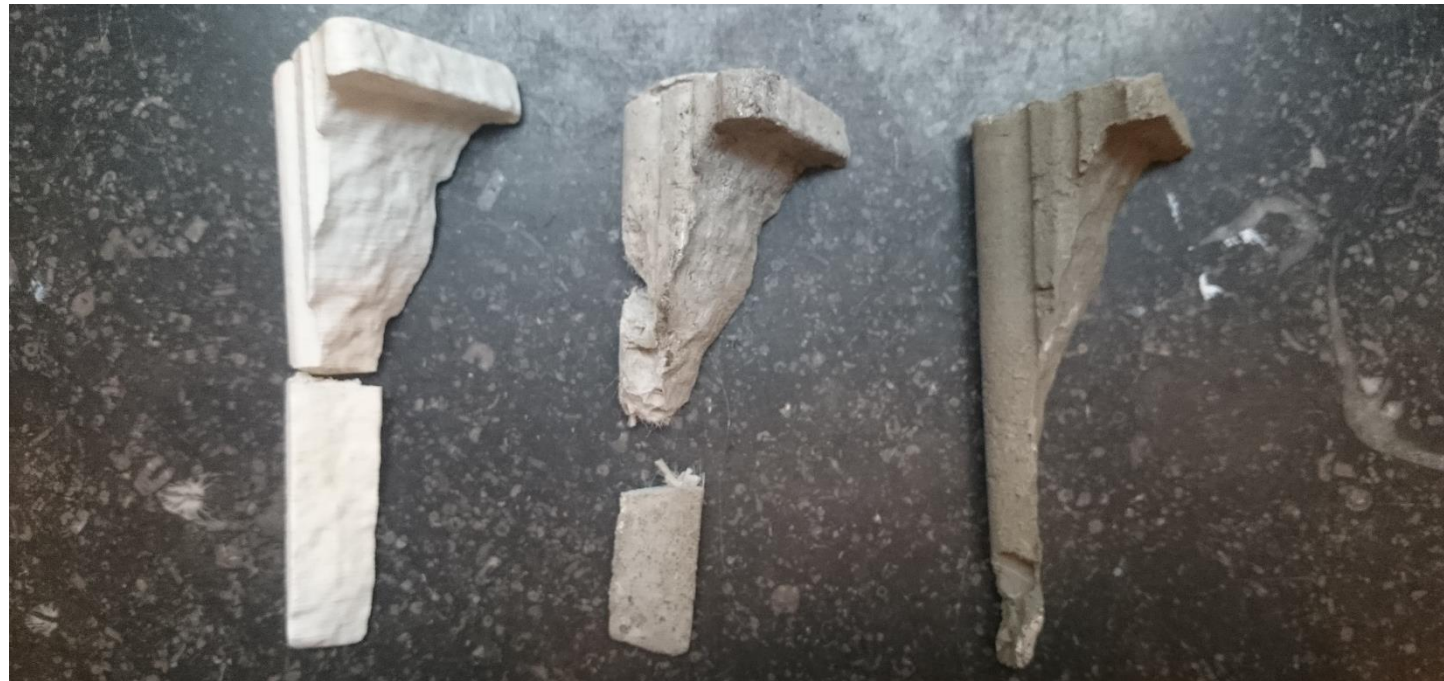
3D Print | Ultracem with lightening pigment and glass fibers | Just Ultracem
