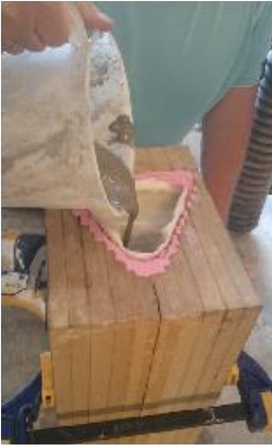
The setup was placed on a vibrating table and the casting material (cement or cement and aggregate) poured
