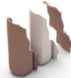
The ceramic 'investment' needs to be dried for 1-2 days before use.
