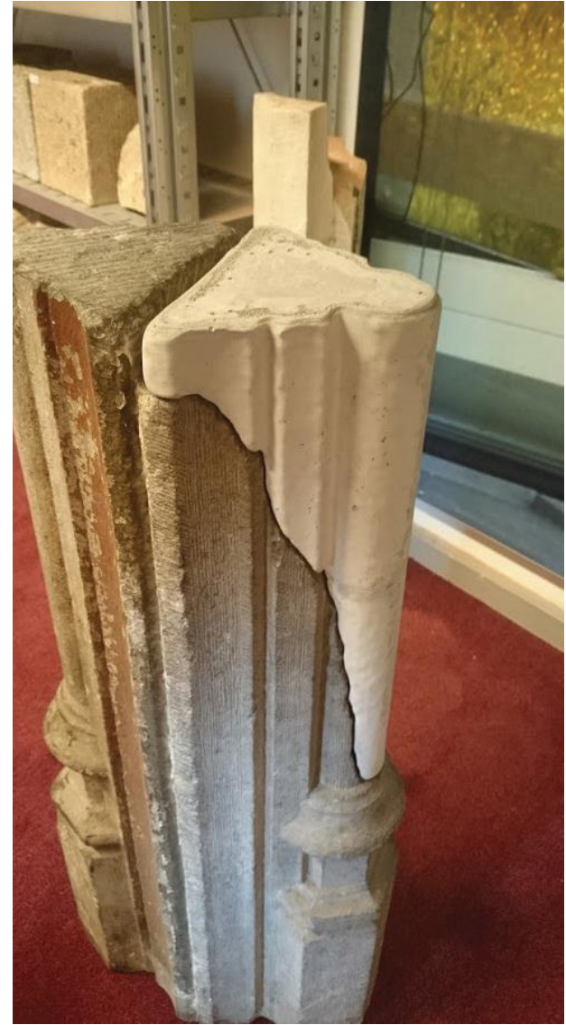
Second cast (with aggregate and 20 g white pigment)
