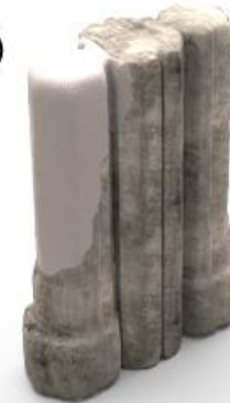
The ceramic mold is then used to cast the cement addition.
