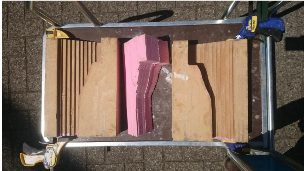
The silicone was released from the reinforcement
