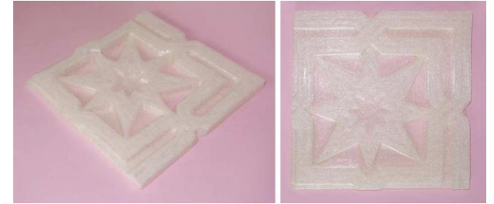
Fused Deposition Modeling (FDM) - PLA material (Low quality but cheap)
