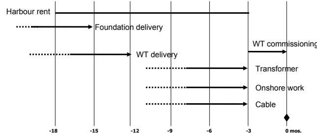
Figure 6.9: Runtimes for an offshore wind farm used in the model. Based on the time to finish for the park, the main contractor determines end times for the various parts of the park.
