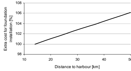
Figure 6.17: Foundation installation cost versus the distance to the harbour. The costs for a park at the same distance as OWEZ are set at 100 %.
