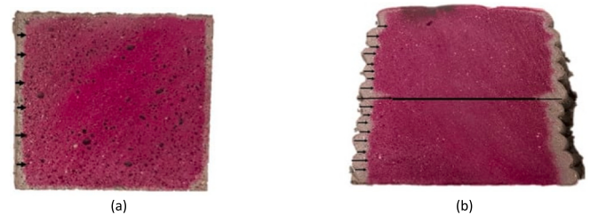
Fig. 8. Determining carbonation ingress depth on (a) mold cast and (b) printed concrete samples (taken from [57]).
