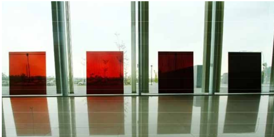
FIG. 5.17 Transparent and coloured PV modules via modification of the Cell thickness (Tsai, 2020).
