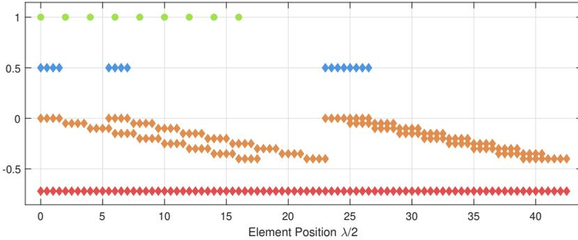
Figure 4.1: Sensor layout of the TI cascade evaluation board. The Tx sensors (green, spaced by  $2\lambda$ ) and the Rx sensors (blue) form a MIMO array with a lot of overlapping sensors. The final 86 unique sensor positions are marked in red.
