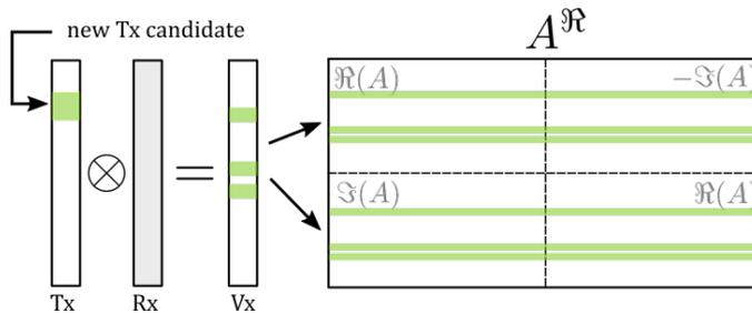
Figure 3.5: Exemplary illustration of the relation between new sensors in the Tx MIMO array, resulting new sensors in the virtual array and finally new rows in the expanded steering matrix. The Rx MIMO array is considered unchanged in this example.
