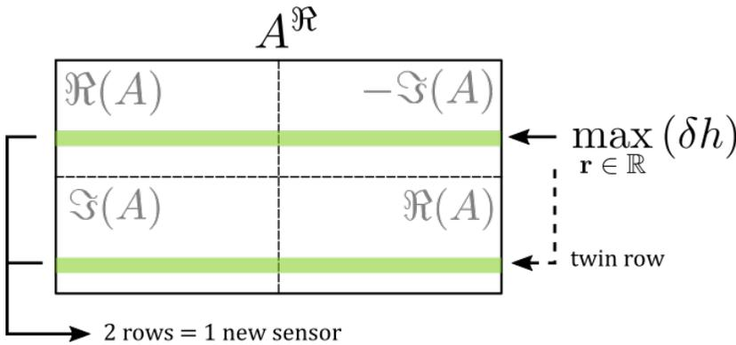
Figure 3.2: Conceptual visualization of the relationship between sensor elements and rows in the expanded steering matrix. The upper row is the one for which the entropy update equation achieves a maximum. However, adding the corresponding sensor will add the lower row as well due to the matrix expansion from a complex to a real valued one.
