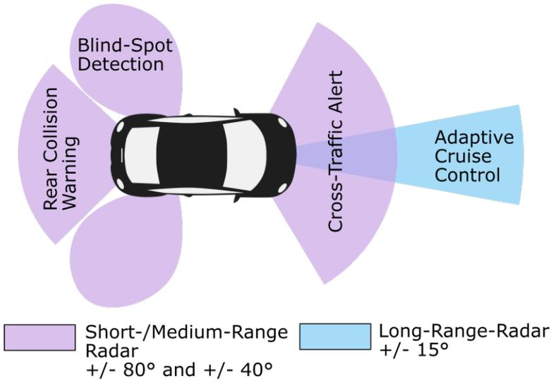
Figure 1.1: Short to long range radar in the automotive industry. Note the use of larger field of views for the short range radar (red) and a rather small field of view for the long range radar (blue). Image derived from [7]
