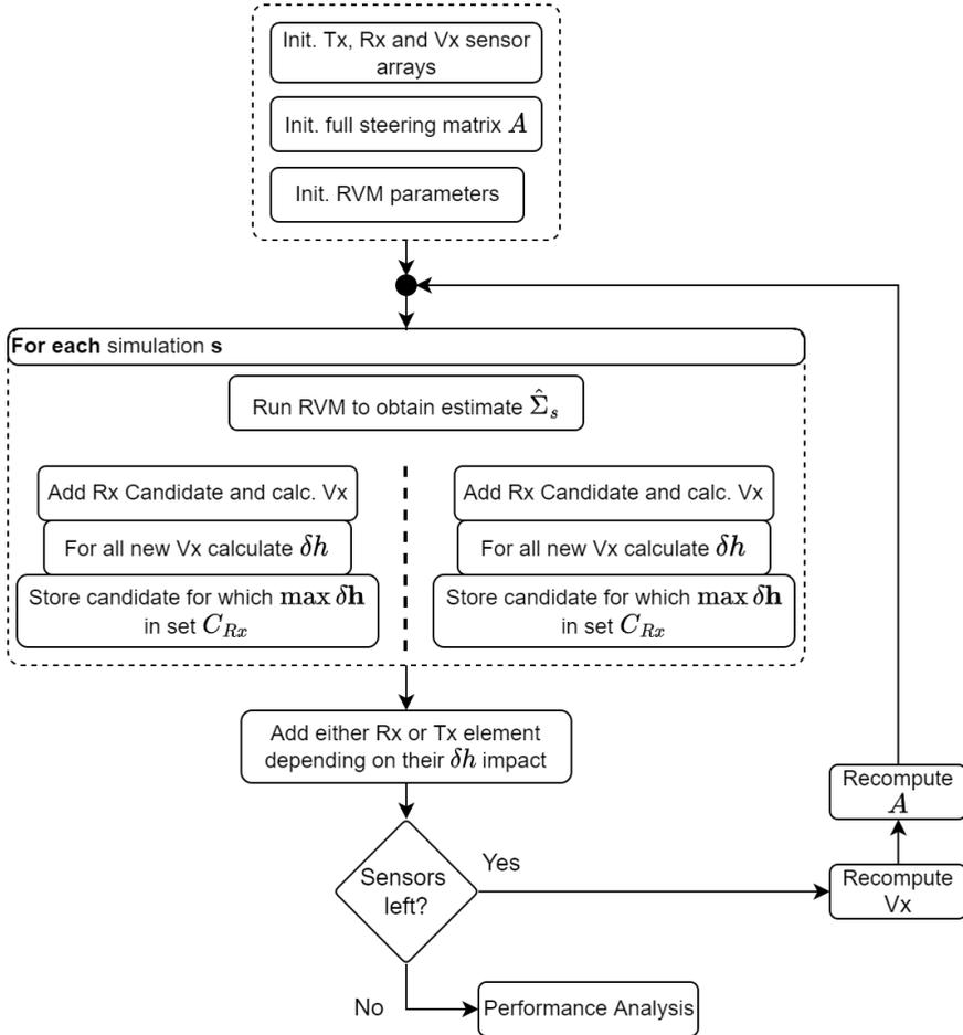
Figure 3.4: Overview block diagram of the entropy based sensor inclusion algorithm for the MIMO case.
