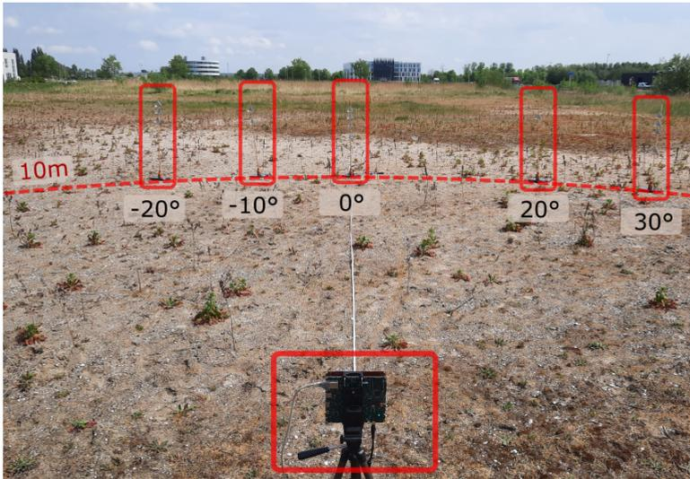
Figure 4.3: Measurement scene from the Radar point of view. All four maximally used targets have been placed at the 10m range from the radar at the angles -20°, -10°, 0°, 20° and 30°.
