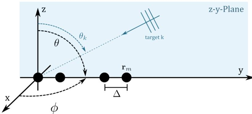
Figure 2.2: Incident plane of target return signals and sensor placement into a linear array. An exemplary target is shown with its incident angle denoted as  $\theta_k$
