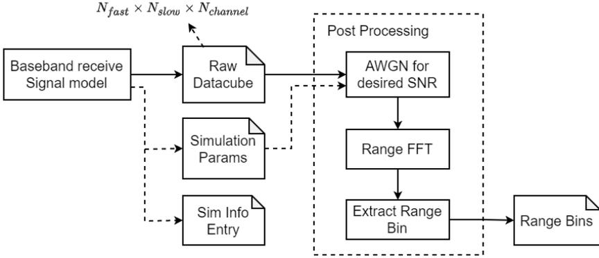
Figure 2.5: Block diagram of the simulation used in this thesis for received FMCW MIMO baseband signals based on the model that has been described in this chapter.
