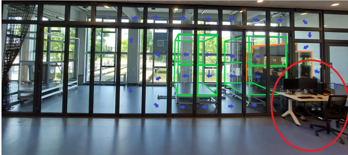
Figure 3.1: Overview of the DCSC Wind AI facility. The WindShaper fan wall (highlighted in orange) generates custom wind profiles within the modular wind tunnel sections (green), which can be extended or reconfigured as needed. The test section is located behind the black windows, while the operator workstation is circled in red on the right. Blue arrows show the airflow path: wind is blown through the tunnel and recirculated back along the top and sides of the facility.
