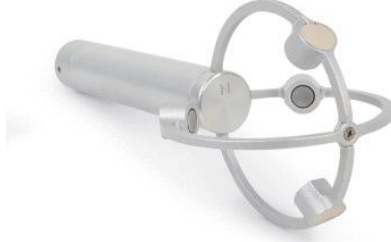
Figure 3.3: TriSonica ultrasonic anemometer with four transducers in a tetrahedral arrangement. It measures three-dimensional wind speed and direction by analyzing the time-of-flight of ultrasonic pulses along multiple axes [47].
