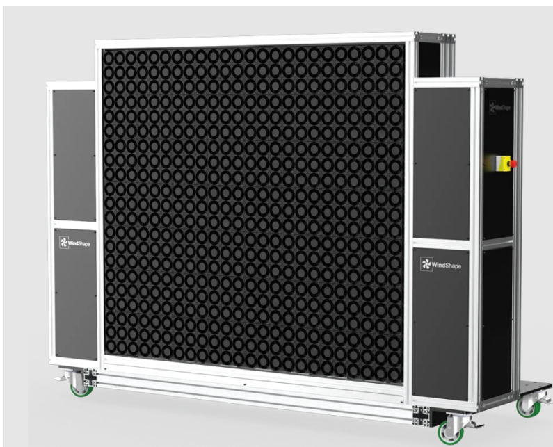
Figure 3.2: The WindShaper uses a modular fan array to generate complex inflow patterns by selectively activating fans. Accurate spatial and temporal flow assessment is essential for validating experimental conditions [37].
