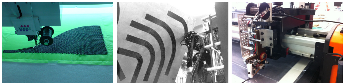
Figure 2.2: Manufacturing technologies for VSL production, from the left to the right: TFP [23], AFP [27] and CTS [31].
