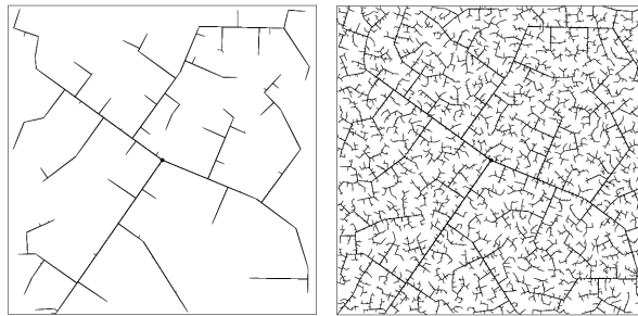
Figure 2.10: Representation of RRT graph trees after 45 iterations and 2345 iterations. Cited in [54], p.230.
