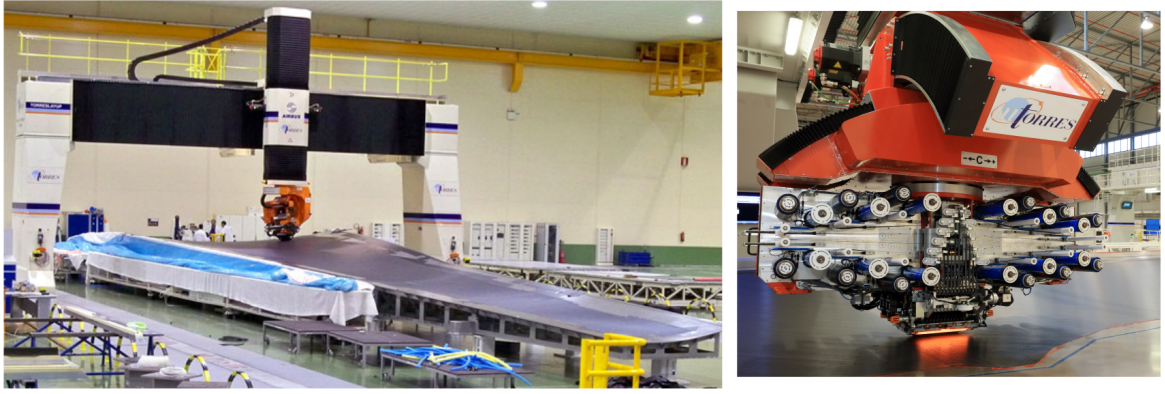
Figure 1.3: Example of an industrial ATL/AFP system: at the left a high-rail TORRESFIBERLAYUP of MTorres used by Airbus and at the right its large deposition tool for high productivity. Copyrights MTorres.
