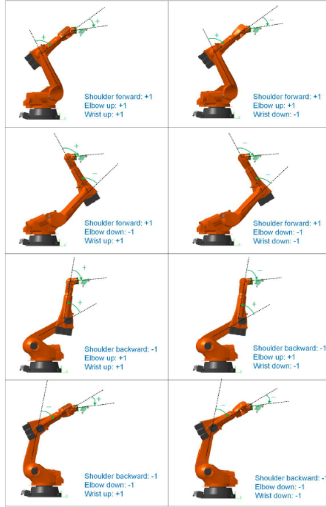
Figure A.4: Eight possible robot configuration for the same end-effector pose. Cited in [10], p. 40.
