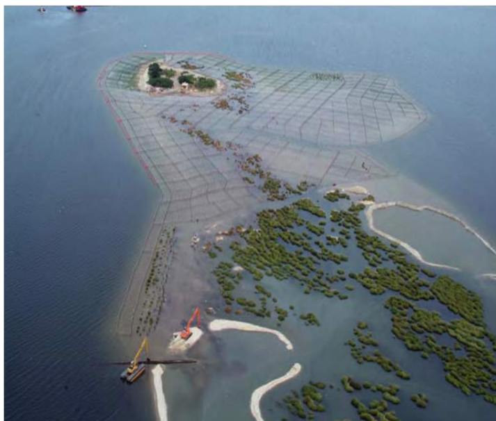
Figure 10.10: Restoration of Elders West using sand berm (USACE [63])
