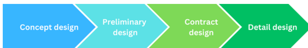
Figure 2.1: Ship design process as described by Gale [30]
