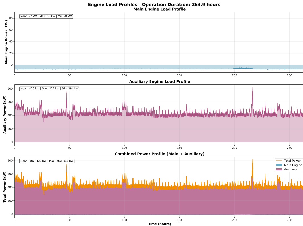
Figure 6.9: Loitering near port load profile.
