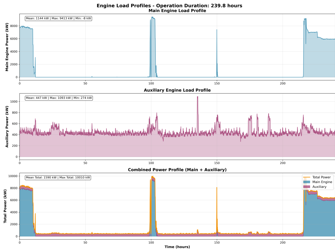
Figure 6.8: Port operation load profile.
