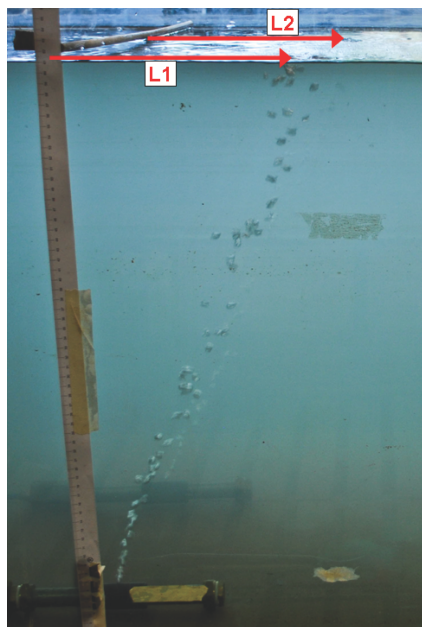
Figure 2.4: Side view of the measurements in the laboratory flume; L1 represents the horizontal displacement of bubbles originating from the nozzle located near the flume's wall, L2 of the ones from the nozzle located in the middle.
