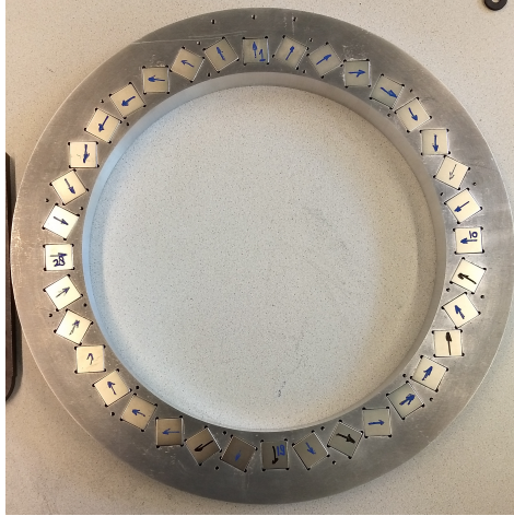
Figure 11: Outer gradient ring existing of 36 1-inch cube NdFeB N52 magnets in a second order Halbach configuration with a radius of 0.175 m.
