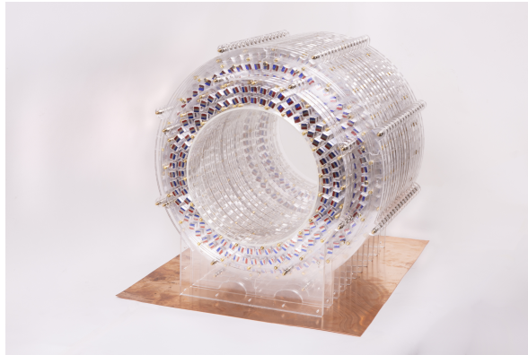
Figure 1: Latest version of the low field MRI-scanner prototype that is made in Leiden [4].
