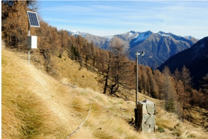
Figure C-3. Picture of the Precipitable Water Vapor Monitor
