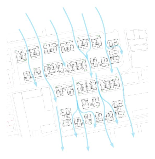
The wet season in Mumbai is also when the wind is the stronger, as the diagrams indicates high wind speed in the months of March to July. In a tropical climate of Mumbai, wind will play an essential role in cooling inside the unit as well as improving its cross ventilation.
