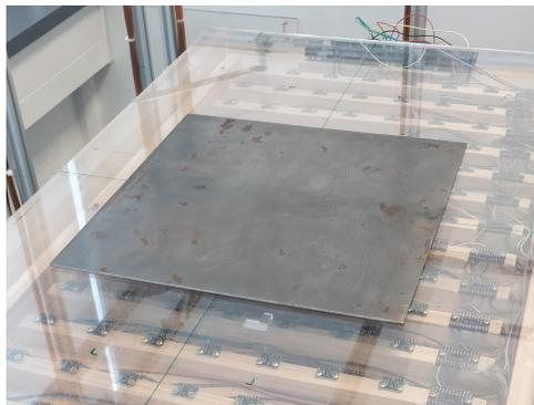
Figuur 5.6: Steel plate above sensor array.
