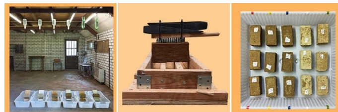
Figure 4 Experimenting with natural binders for rammed earth construction brought about a lack of established protocols for testing rammed earth in the NL. The graduation thesis of Fieke Konijnenberg (2024) identified a series of potential natural binders as well as a clear set of testing protocols based on archival research, literature review, and interviews.
