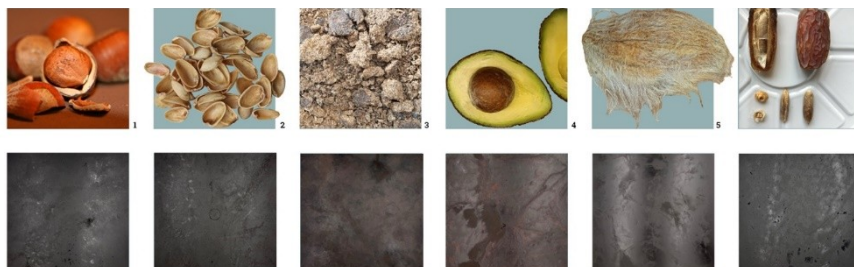
Figure 8 Food-waste streams mapping, and material sampling using the food-streams as fillers and a 98% biobased resin.
