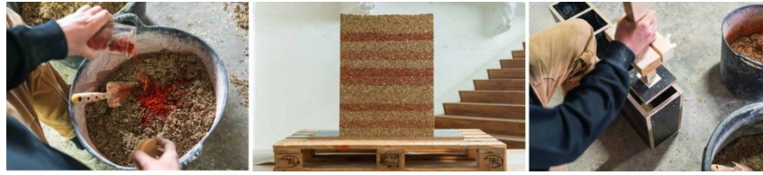
Figure 6 The graduation thesis of Tom Boom (2025) on hempcrete construction research with varying manufacturing parameters such as layer height, compaction factor, orientation and binder type.
