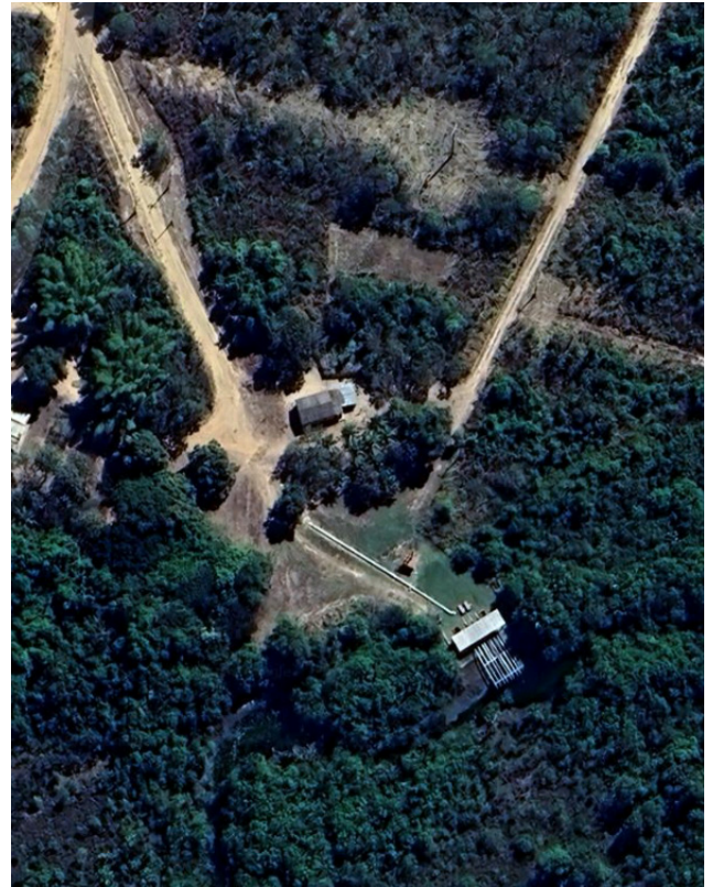
Image 2.14 Water pumping station connected to the river. The infrastructure captures water directly from the river, pumping it into reservoirs that support irrigation systems.
