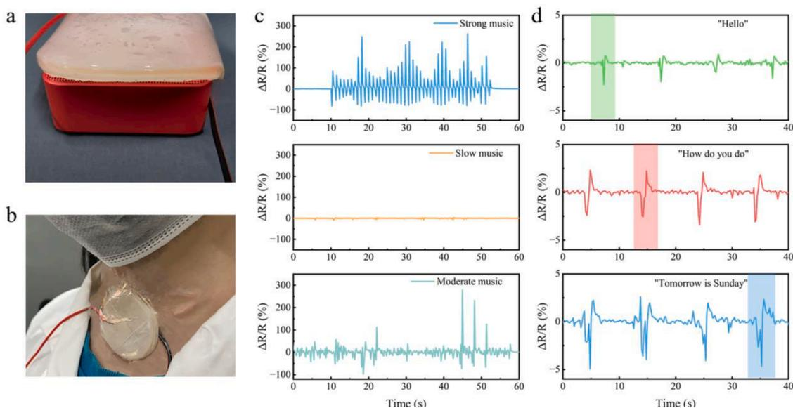
**Fig. 6.** Responses of the -H-C-L-A-H device to various music rhythms and human speaking. The photo of the actual test in responses to various music rhythms (a) and human speaking (b). The relative change of the resistance with the vibrations of different music rhythms (c) and human speaking movements of the throat (d). Each gel round piece was 2 mm thickness and 10 cm diameter (a-d).
