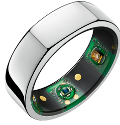
Figure 3.8: The Oura Ring and its PPG sensors. Courtesy of [75].
