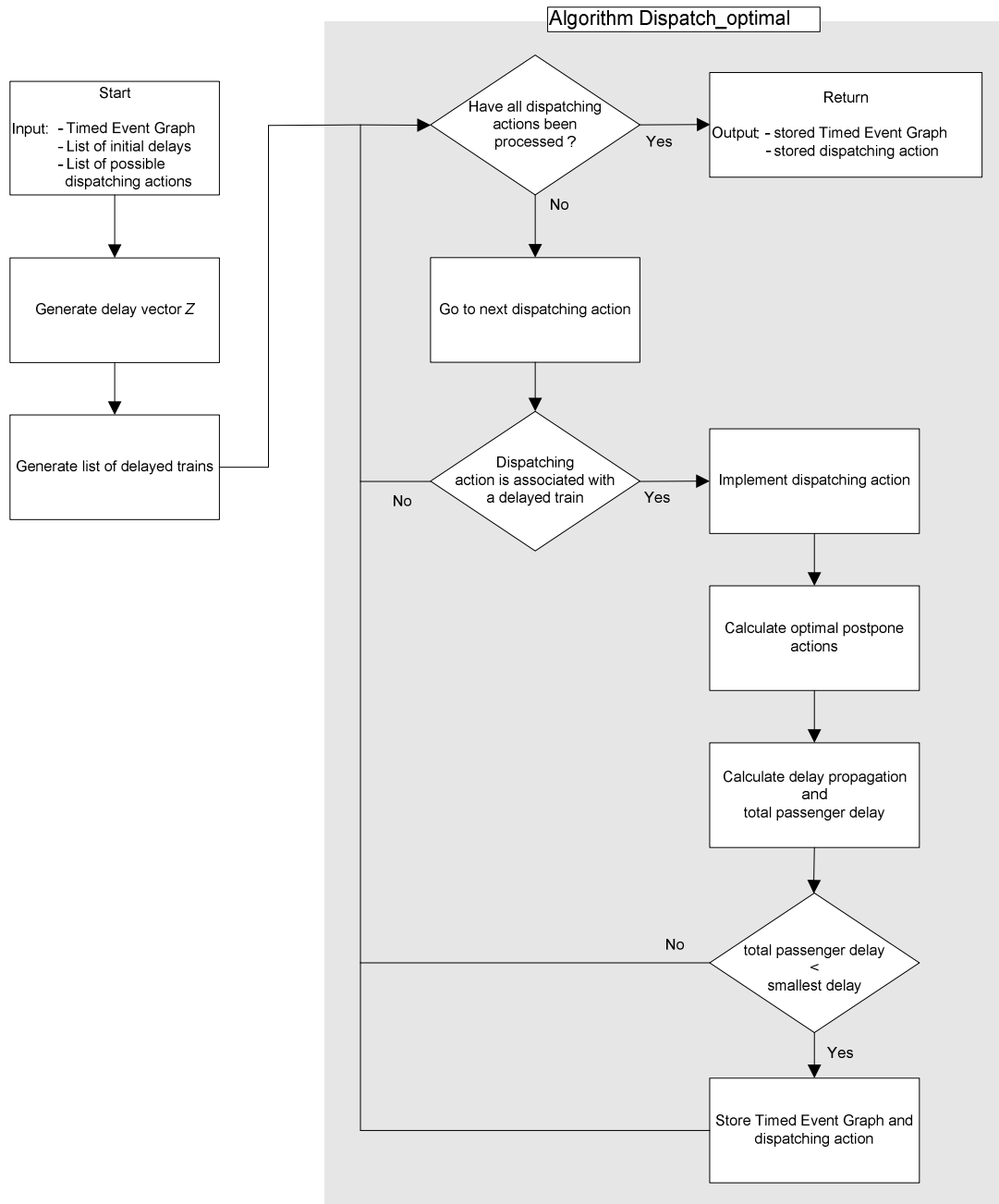
Figure 6.16 Diagram of algorithm 'Dispatch_optimal' to find the most effective dispatching action.
