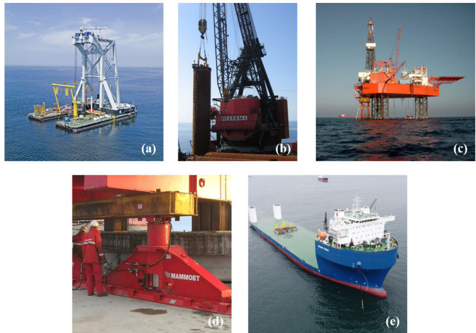
Fig. 14 Traditional offshore erection techniques: a crane vessel transportation also used for pile driving (van de Burg 2006), b suction pile technology (BoH 2006), c common offshore jack-up rig (Mirafori 2010), d skidding equipment mounted on a vessel (Mammoet nd), and e characteristic vessel for FLO-FLO (Seaway 7 nd)
