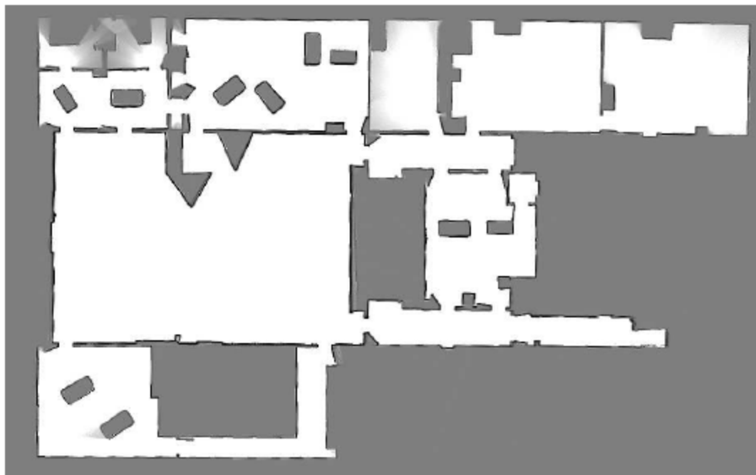
Figure 2.6: An occupancy grid map: the black cells represent detected objects, the white cells represent free space and the grey cells represent unknown/unexplored area [4].
