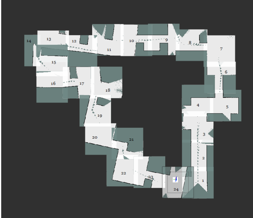
Figure 5.2: Resulting map of the non-hierarchical scheme. When the robot left node 23, it should have traversed back to node 1 but instead it created node 24. Thus, the loop was not closed.
