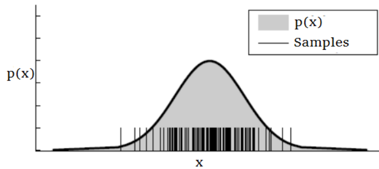
Figure C.1: Particle filter representation of a Gaussian distribution. The distribution is approximated by particles. The area where the particle population is dense depicts high probability of occurrence [2].
