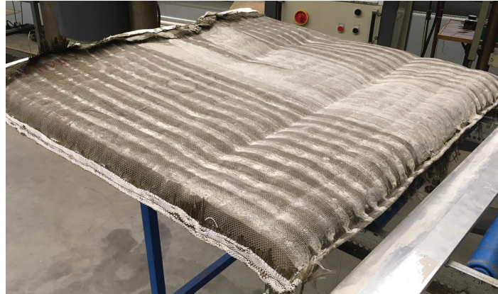
FIG. 13 First demonstrator made of single-curved basalt spacer fabric
