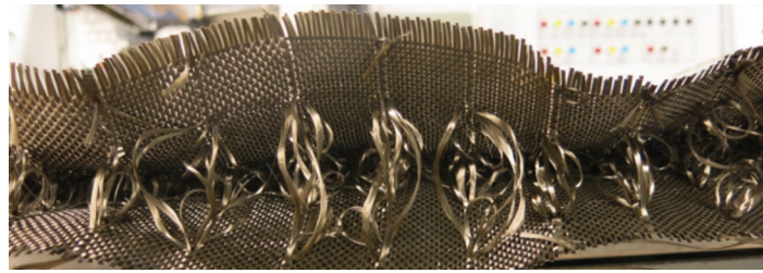
FIG. 12 First-time production of a double-curved spacer fabric made of basalt rovings
