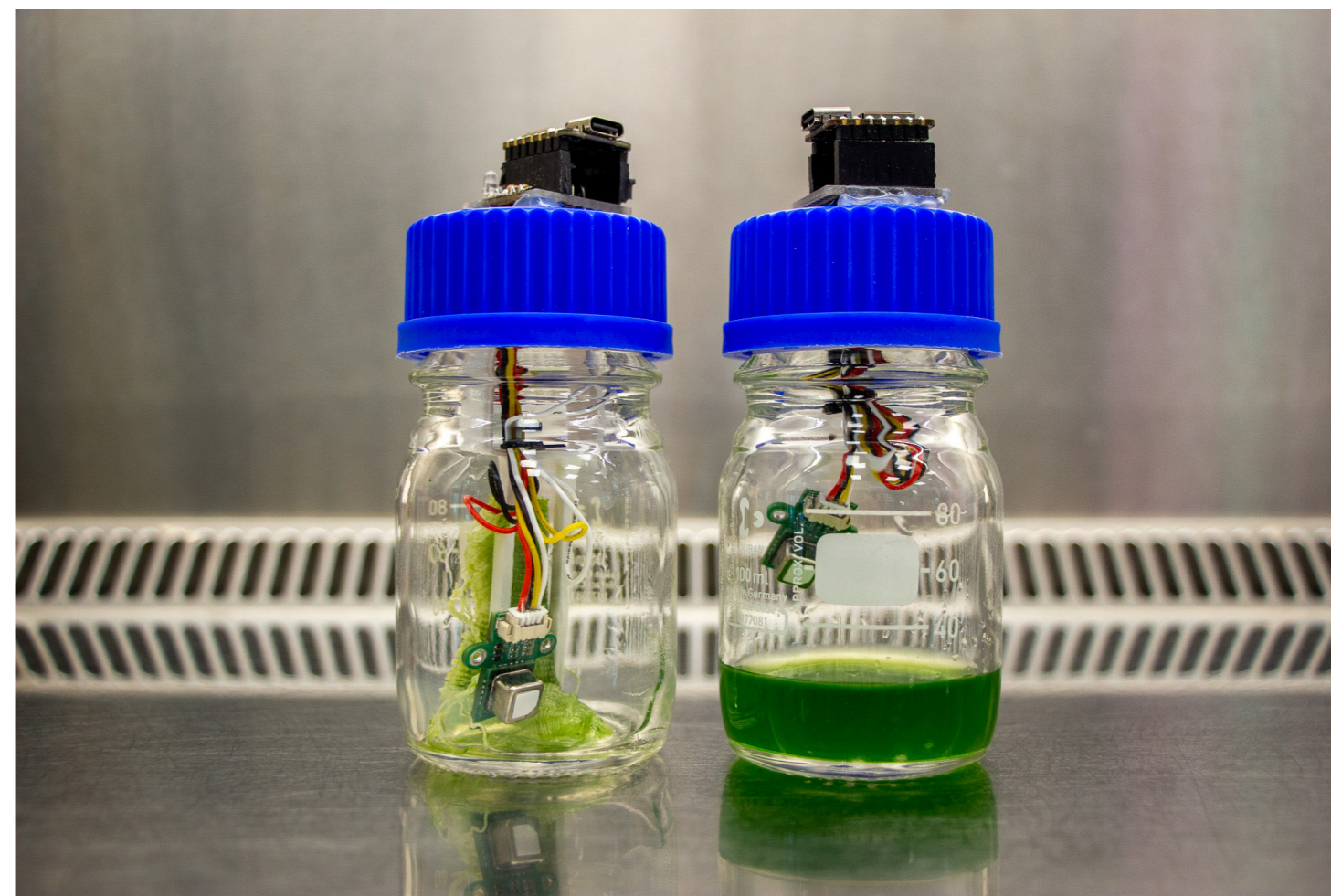
Figure 66: Optimised CO 2 measurement setup with suspended sensors for both microalgae-textile biocomposites and suspension cultures, with samples showing high pigmentation indicative of high viability.
