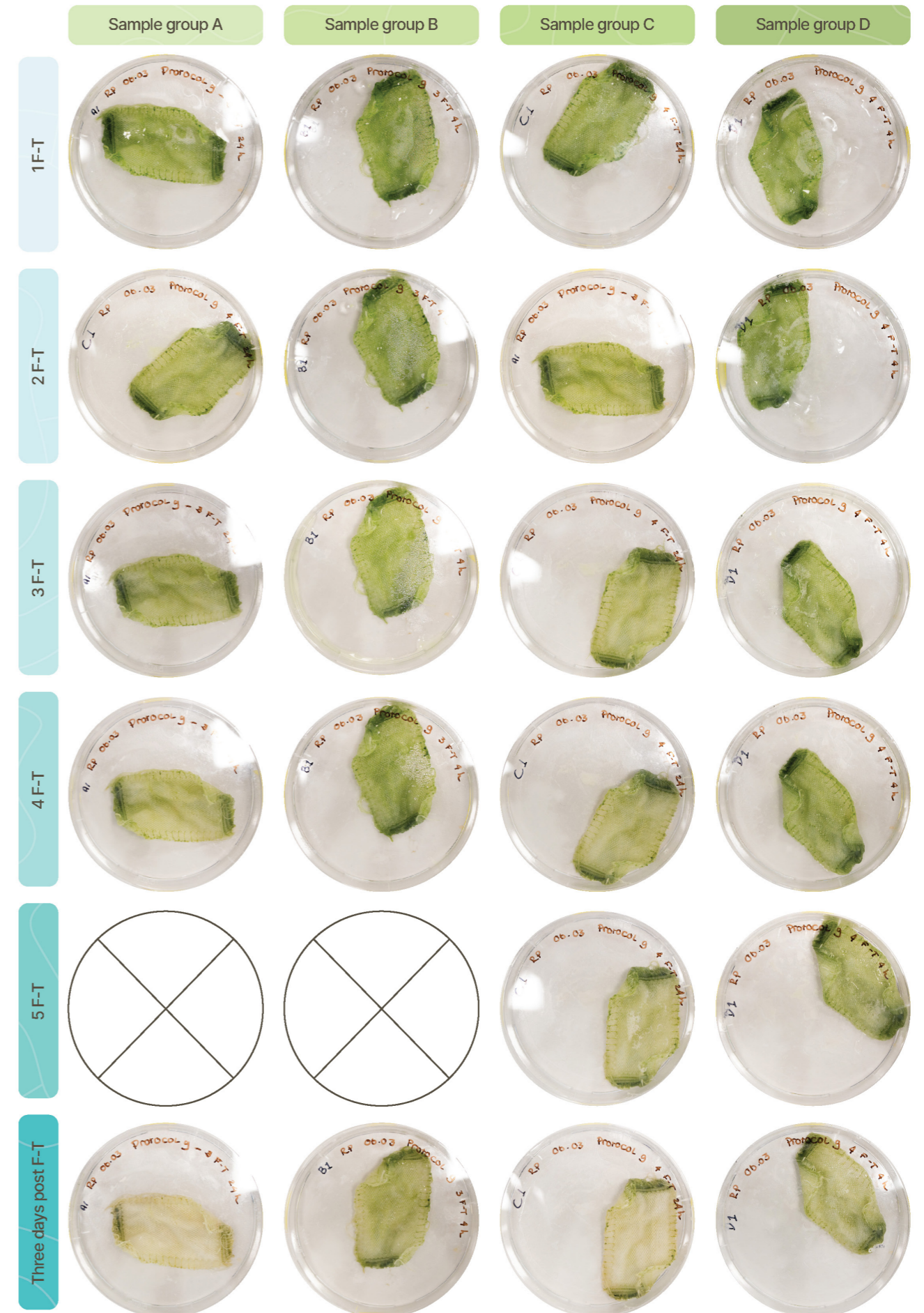
Figure 41: Overview of freeze-thaw samples during thawing. A single representative biological replicate was selected from each sample group for imaging. Sample groups B and D show a less rapid decline in pigmentation compared to sample groups A and C.
