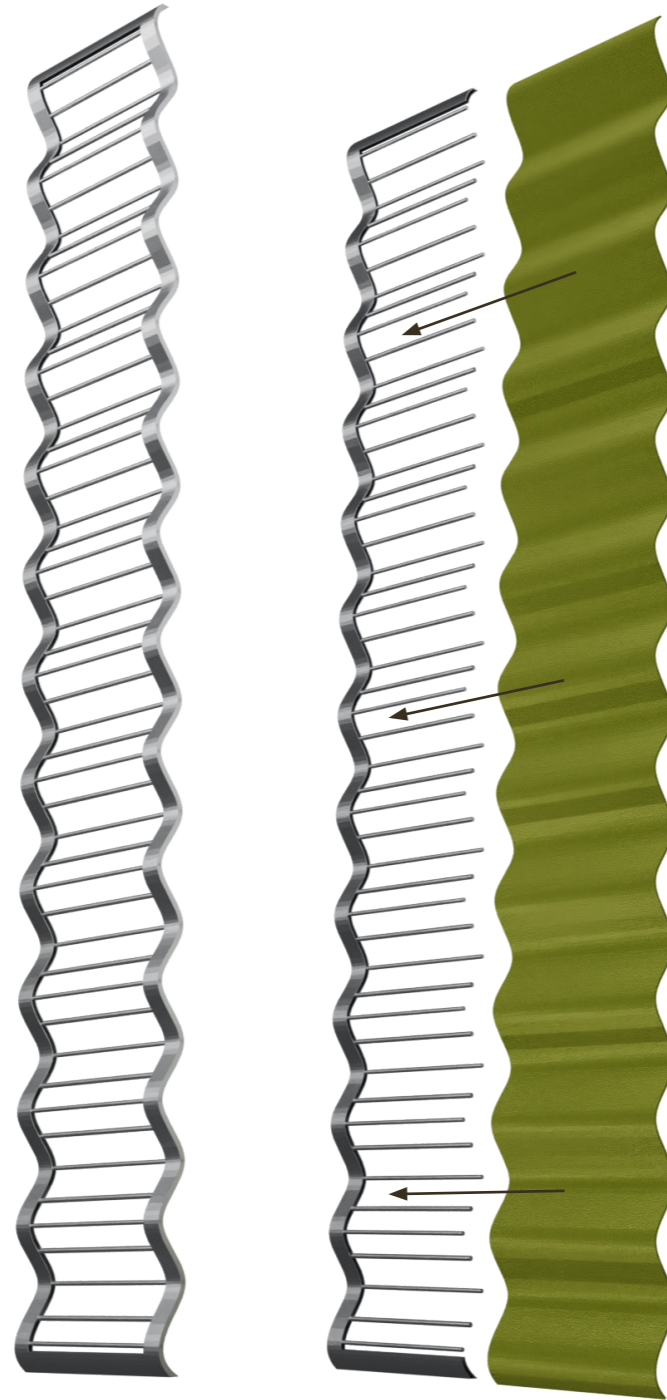
Figure 72: Stainless steel frame supporting the microalgae-textile biocomposite, secured by vertical rods. The integrated channels within the woven structure allow the textile to be tensioned across the rods.
