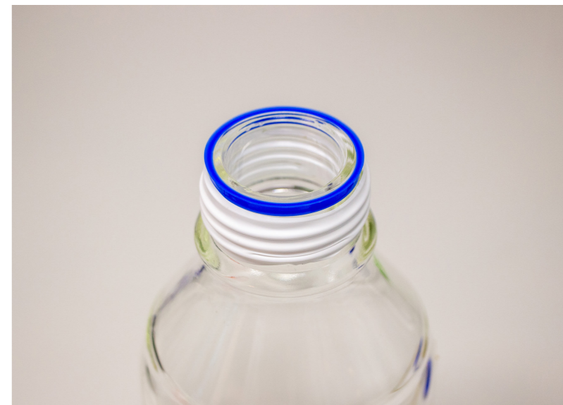
Figure 13: Measurement bottle sealed with PTFE tape and an integrated sealing ring to ensure a gas-tight CO 2 measurement environment.
