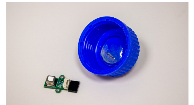
Figure 7: Cap of the CO 2 measurement setup featuring a detachable CO 2 sensor to enable sterilisation.
