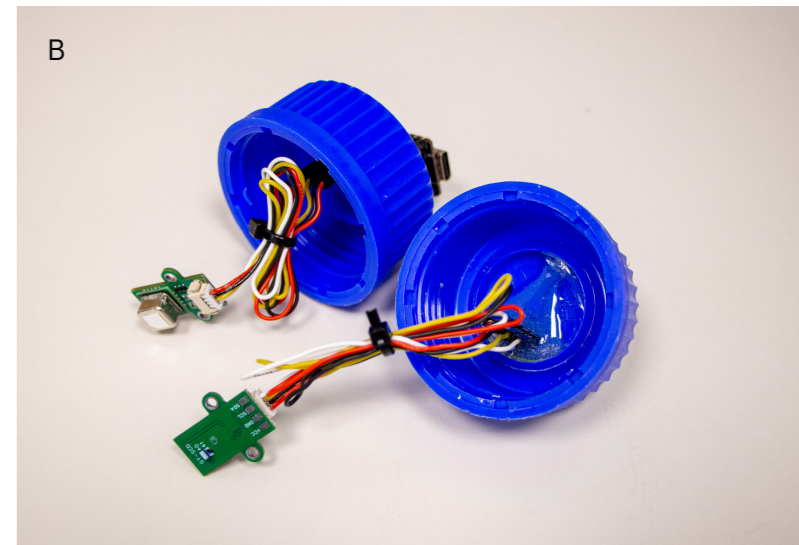
Figure 12: (A) Initial CO 2 measurement cap with integrated sensor; (B) final design with suspended sensors for both textile samples and suspension cultures.
