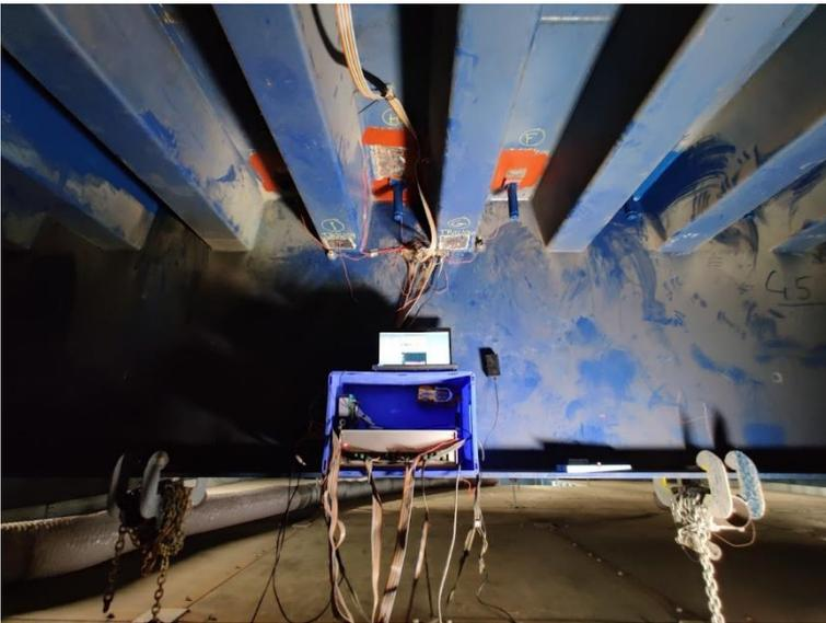
**Figure 48: Measuring equipment setup (picture taken after strengthening)**
