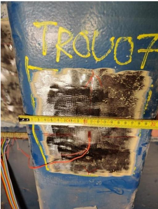
**Figure 49: location of sensor TROU07, approximately 5 mm off-centre**
