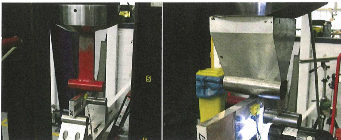
Figure 5.16: Improvement of the 3 point bending setup by replacing the T-shaped cylinder (left) by a rigid block.
