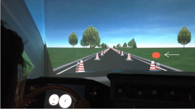
Fig. 2: Visual warning when a cone is hit: a red light appears on the side of the steer where the car left the road (indicated here by white arrow).
