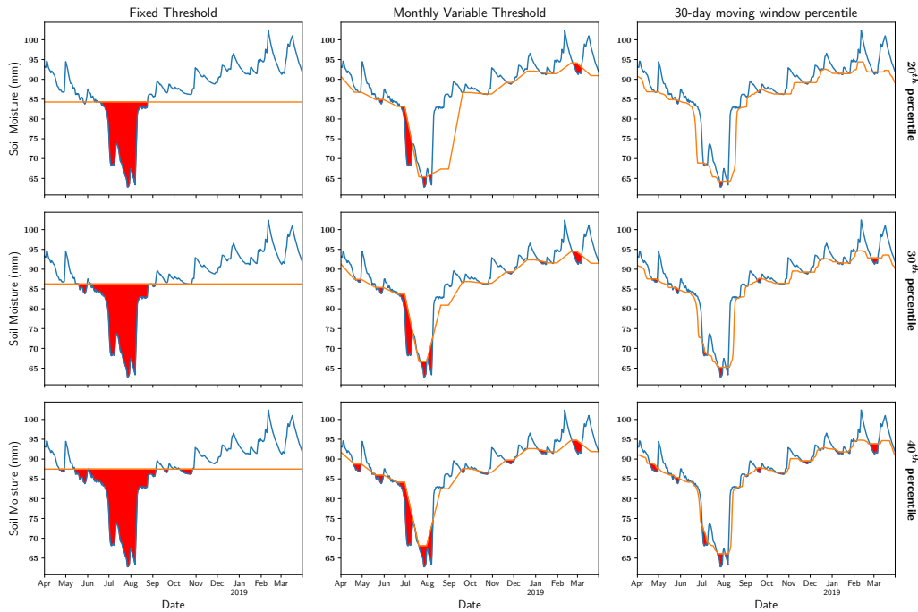
Figure 4.19: Soil moisture drought events identified using fixed, variable, and moving window threshold for three different percentiles for well L-PB46 in district w_0
