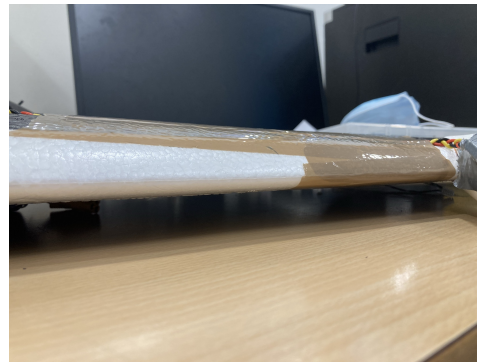
Figure 3.3: Improved motor wire layout, designed to restore the wing profile.
