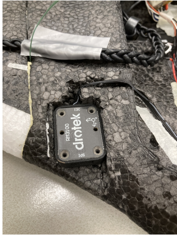
Figure 3.16: Original placement of RM3100 magnetometer sensor, on the leading edge at the wing root. The proximity to the motor wire was causing interference.
