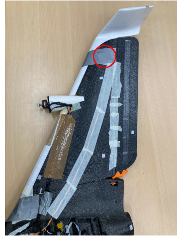
Figure 3.17: Wingtip placement of RM3100 sensor, near the wingtip or the right wing. The larger distance to other electrical components improved performance.
