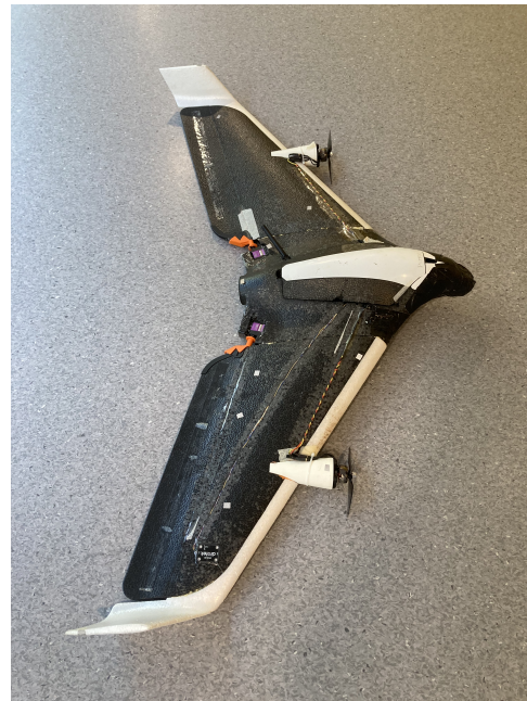
Figure 1. Modified Parrot Disco. The standard pusher motor was replaced with two reversible puller motors to power the flat spin. The nose cone was added to house ballast to shift the center of gravity forward.
