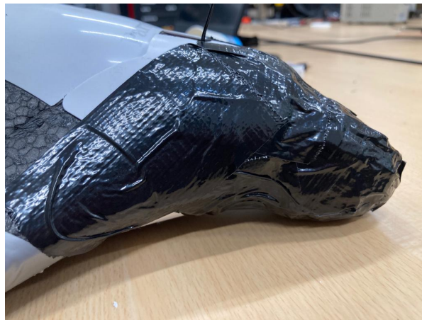
Figure 3.20: Side view of nose cone, added to shift center of gravity forward.
