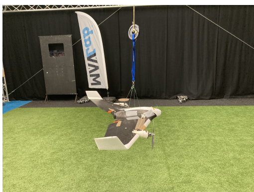
Figure 4.1: First CyberZoo experimental setup. The drone hunged from a hemp rope, using a swivel J-hook from a name tag lanyard holder to allow the drone to rotate.
