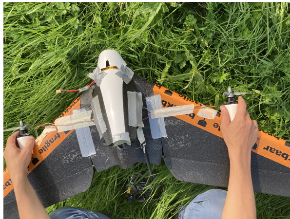
Figure 3.1: Original motor wire layout.
