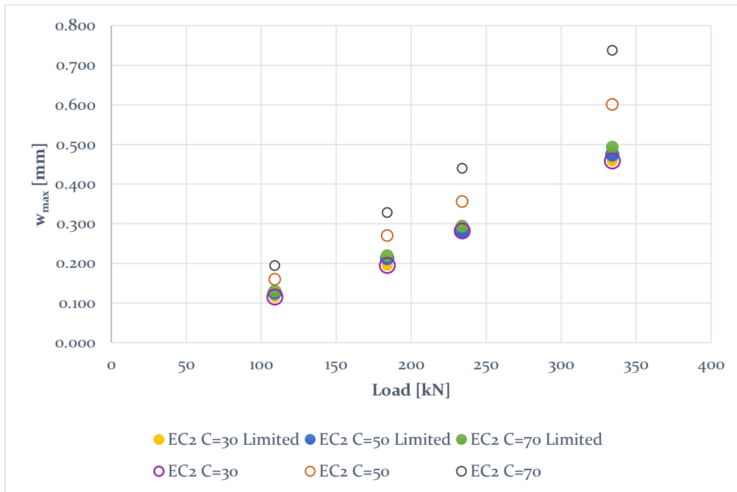
Graph 2-3: Influence of the limitation of the maximum crack spacing on the maximum value of the crack width according to VARCE for Rectangular beam 13
