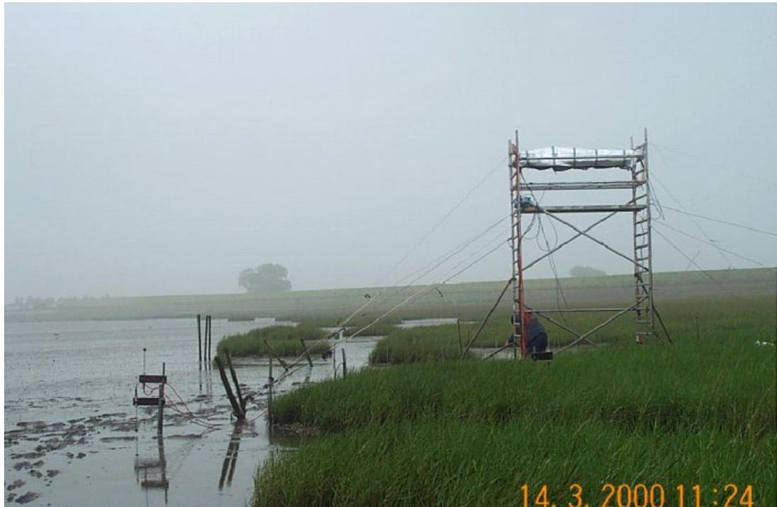
Figure 3.4: A ‘logger tower’ and some gauges near the edge of the salt marsh.
