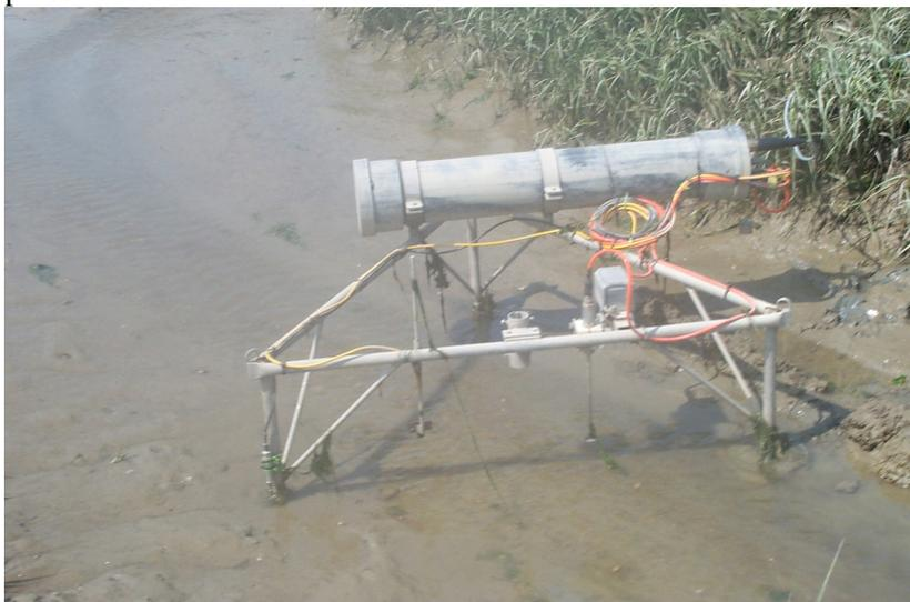
Figure 3.1: Example of measuring frame in the salt marsh creek
