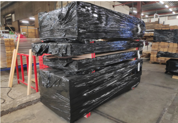
FIGURE 19 Black plastic wrapping used internally and for transport
