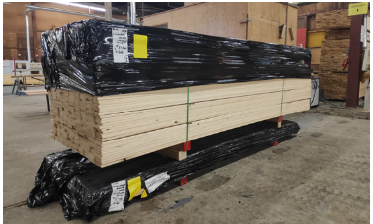
FIGURE 31 Improved situation, only wrapping the top of the pile reducing the material used by more than 50%
