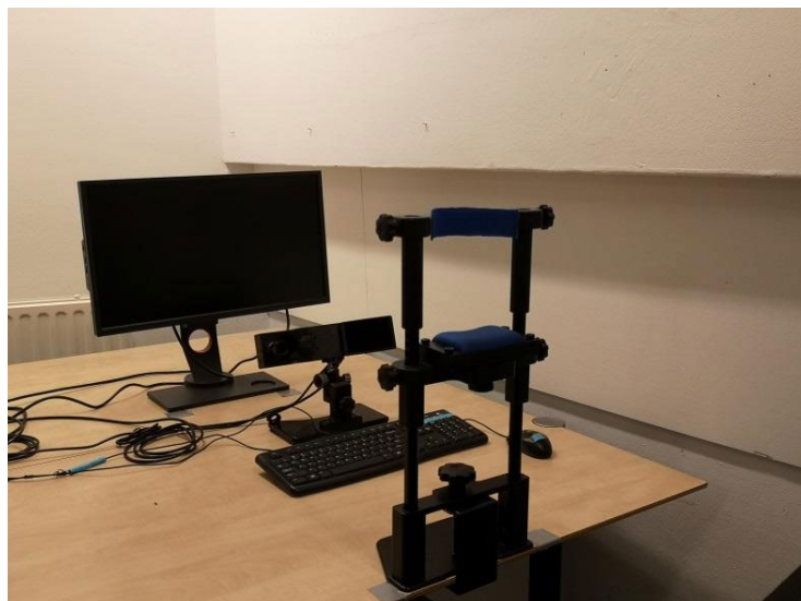
Experimental setup with head support and eye-tracker.
