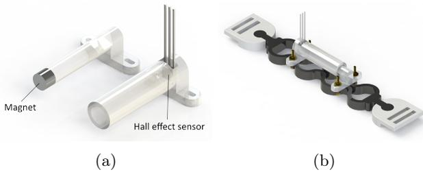
Figure 4: (a) Sensor mounts with magnet and Hall effect sensor. (b) Sensor mounts attached to TPU phantom muscle with brass M1 bolts.
