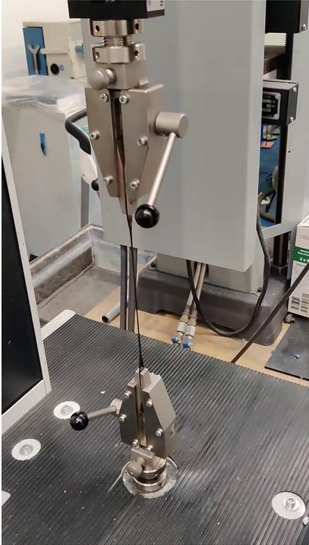
Supplementary figure 16: Tensile test of 3D-printed samples using a Lloyd tensile testing machine.
