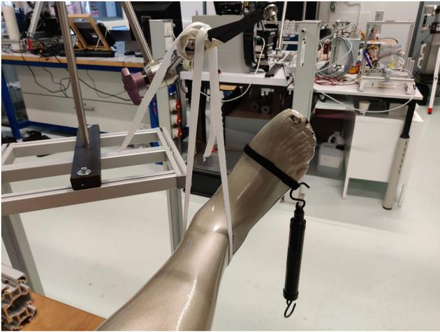
Supplementary figure 13: Ankle is held in place during the additional stability testing.
