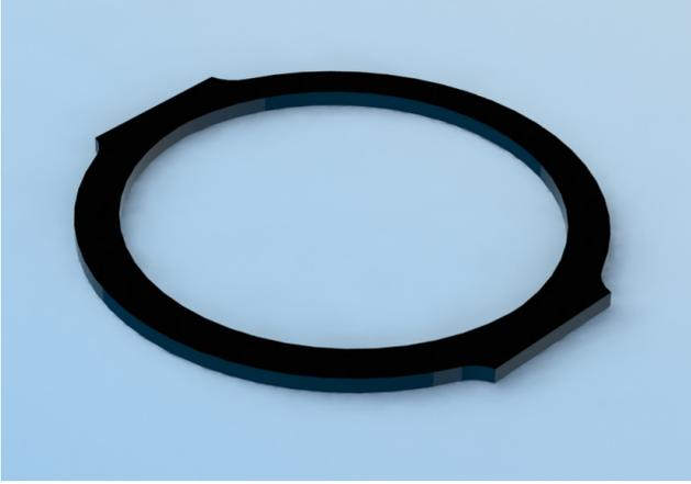
Supplementary figure 5: 3D-render of circular spring concept. A force is applied perpendicular to both square surfaces to create a force with increasing stiffness modulus.
