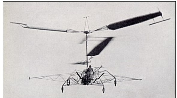
FIGURE 1. CORRADINO D'ASCANIO'S HELICOPTER WITH SERVO TABS.
