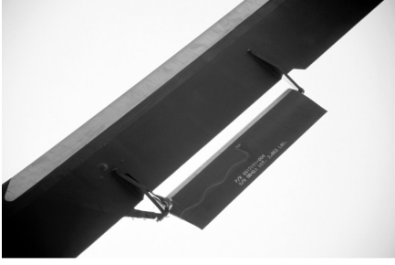
FIGURE 2. FLAP USED IN KAMAN HELICOPTERS.
