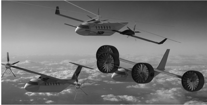
Figure 8.2: Render of the heliplane, TRAC tiltrotor and 4 Ducted Fans concept
