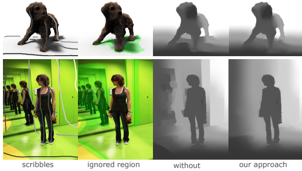
Figure 5: Ignored-gradient region. Shadows and reflections introduce unwanted large gradients, which hinder the depth diffusion and lead to discontinuities. Using the ignored-gradient region brush, these gradients can be excluded from the depth derivation. (Top image: courtesy of Erik Sintorn; bottom image: Flickr - salendron)
