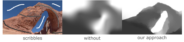
Figure 4: Depth estimation from scribbles. Scribble input (left), only using the scribble input results in a smooth depth map lacking discontinuities (middle), by involving the input image gradients, the depth propagation is improved (right). (Image source: www.pixabay.com )
