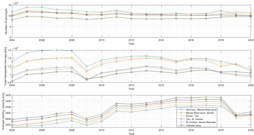
**Figure C.1:** Comparison intensities Waal-Volkerak locks; top panel) number of annual passages, middle panel) total annual transported tonnage, bottom panel) average vessel loading capacity
