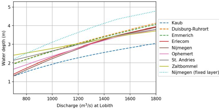
Figure 2.2: Relation between discharge at Lobith and the MGD's measured at several locations along the river Waal and Rhine. Adopted from (De Jong, 2020a)
