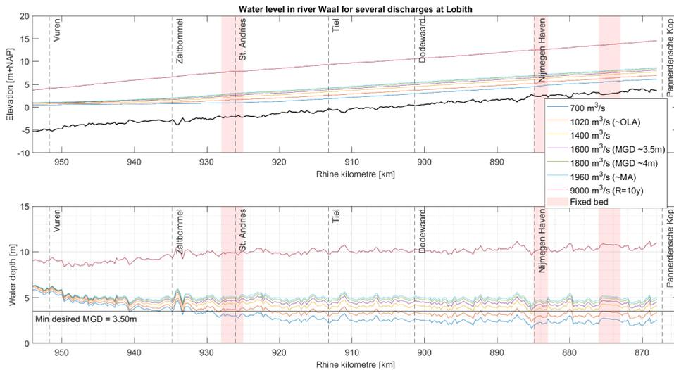
**Figure 3.6: Upper panel:** water levels for several discharges at Lobith, **lower panel:** water depth for several discharges
