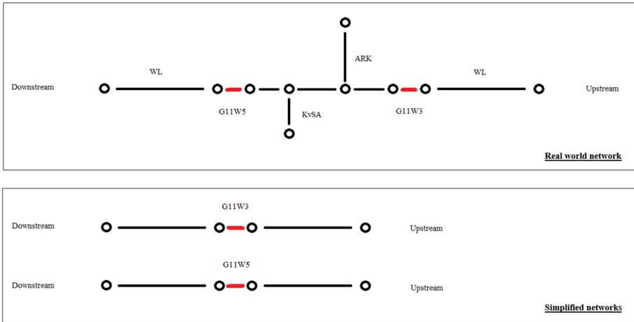
**Figure 4.1: Upper panel:** One network including two lock complexes, **Lower panel:** Two separate networks both including one lock complex (WL = Waal river, ARK = Amsterdam-Rijnkanaal, KvSA = Kanaal van Sint-Andries, G11W3 = upstream lock complex and G11W5 = downstream lock complex)
