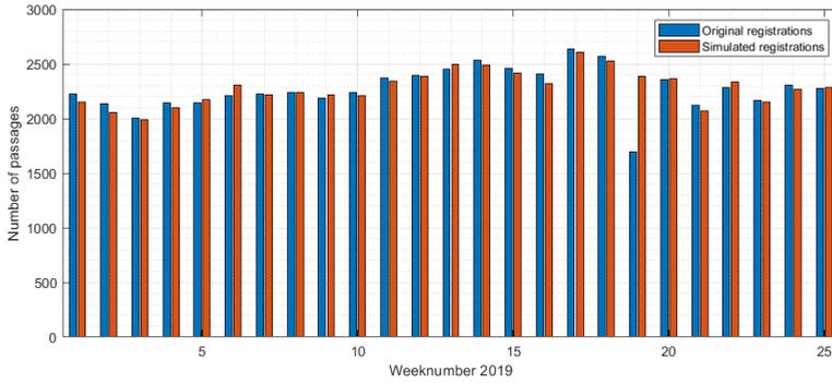
**Figure E.5:** Comparison between original IVS vessel registrations and vessel generation in SIVAK for the four busiest weeks
