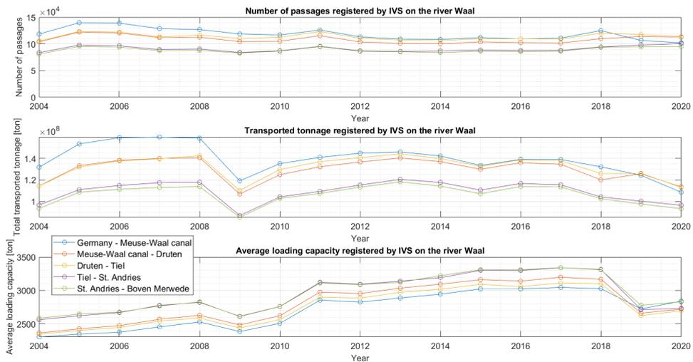
**Figure 2.7:** Annual figures for passages, transported tonnage and average loading capacity on the river Waal. An estimated 10-20% of the vessels is not included in the data. Figures are based on IVS-data.
