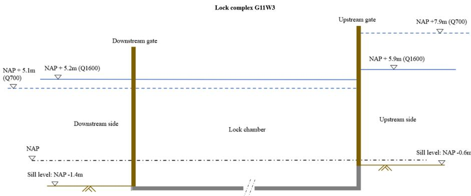
**Figure 4.3:** Longitudinal section of a lock showing normative water levels and sill depths at lock complex G11W3
