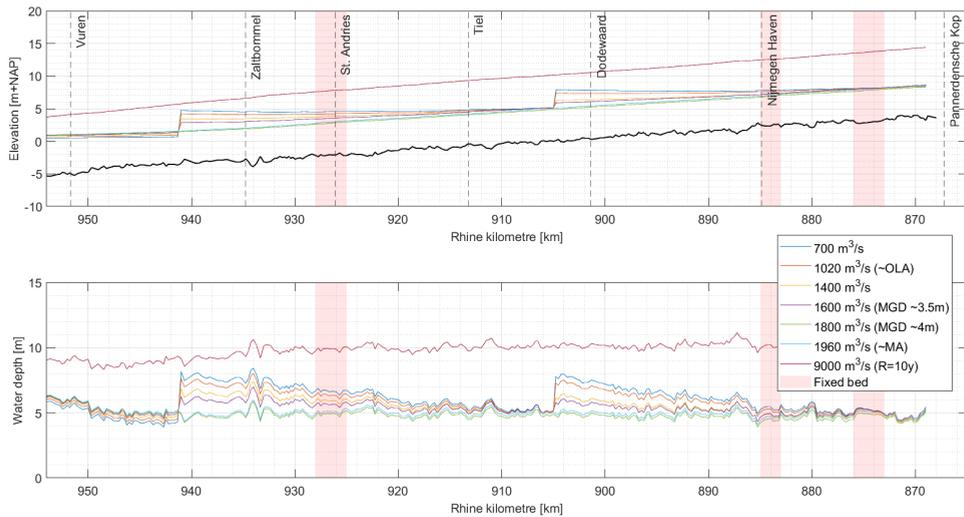
**Figure 3.7:** Upper panel: water levels for several discharges at Lobith, lower panel: water depth for several discharges
