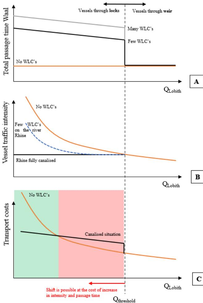
**Figure 3.1:** **Panel A:** relation between passage time Waal and discharge at Lobith for different scenarios, **Panel B:** relation between vessel intensity and discharge at Lobith, **Panel C:** relation between transport costs and discharge at Lobith for the case with and without WLC's (plots are based on (de Jong, 2021))
