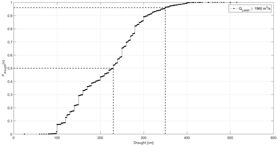
**Figure 3.5:** Empirical cumulative distribution function of the vessels' draught corresponding to discharges larger than  $1960 \text{ m}^3$  at Lobith (based on IVS data between Tiel and Druten 2019).
