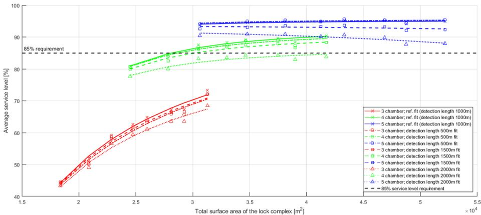
Figure G.7: Average service level for varying detection lengths for model variants at lock complex G11W3
