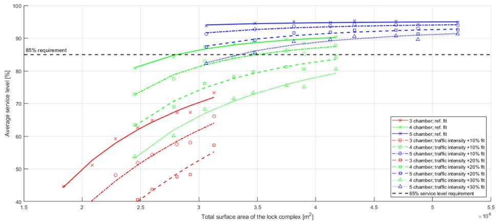
Figure 5.7: Service level for all model variants for varying vessel traffic intensities
