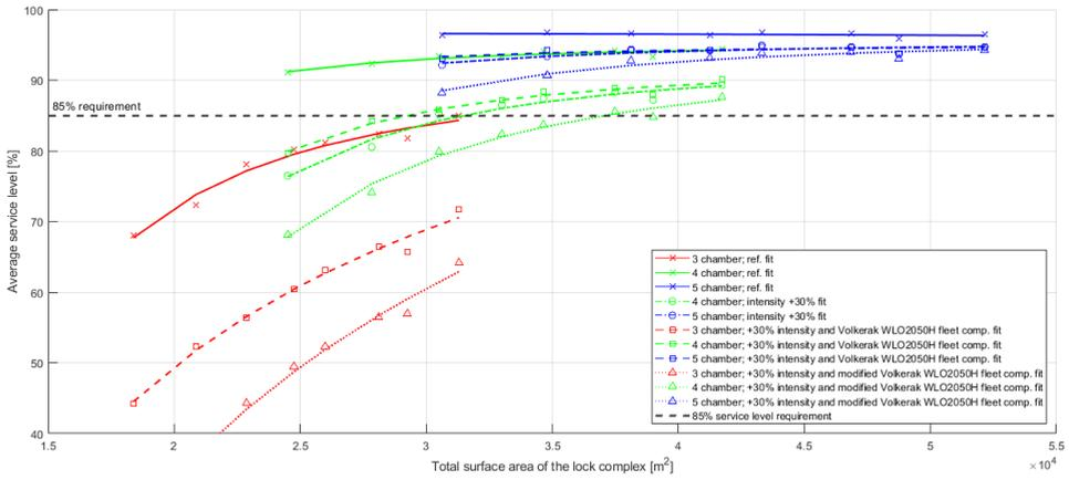
**Figure E.4:** Average service level for all model variants for varying fleet compositions and increased traffic intensity for complex G11W5
