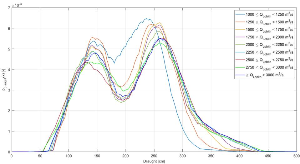
**Figure 3.3:** Draught distribution of vessels passing location G11W3 (Based on IVS data: Jan-Dec 2019)
