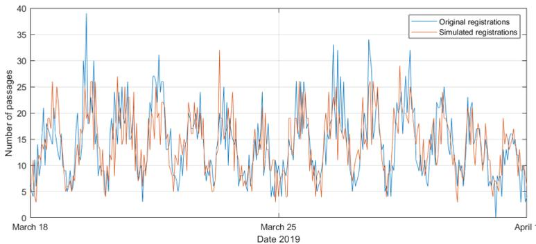
**Figure E.7:** Comparison between original IVS vessel registrations and vessel generation in SIVAK III for the four busiest weeks
