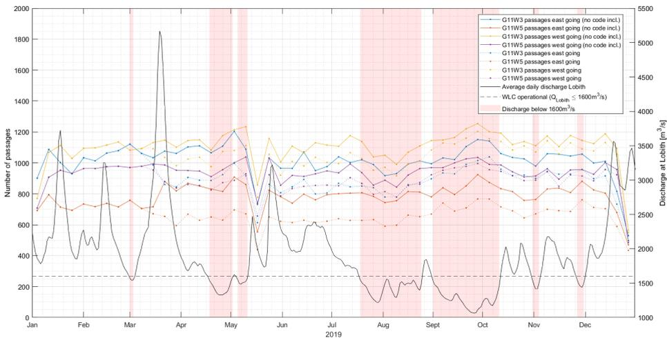
**Figure D.16:** Weekly number of commercial vessel passages at locations G11W3 and G11W5 for 2019 and average daily discharge at Lobith
