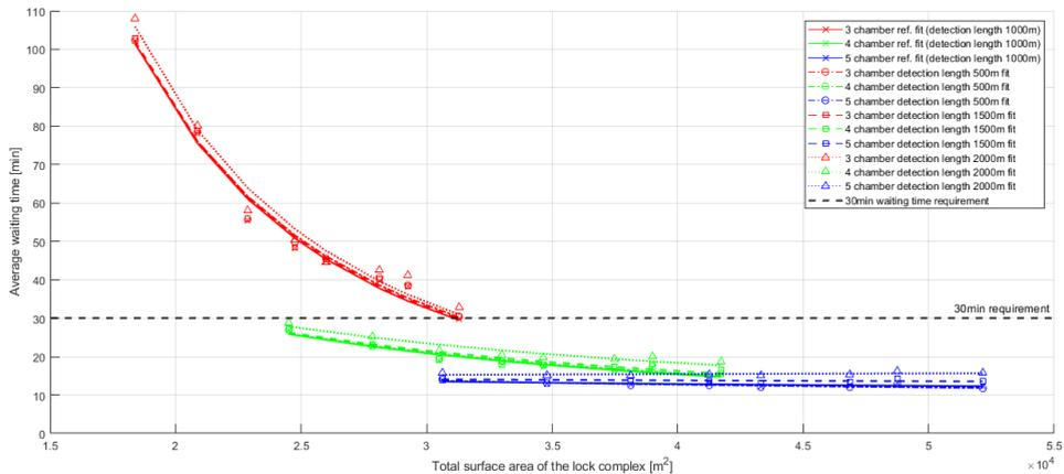
**Figure G.6:** Average waiting time for varying detection lengths and model variants at lock complex G11W3
