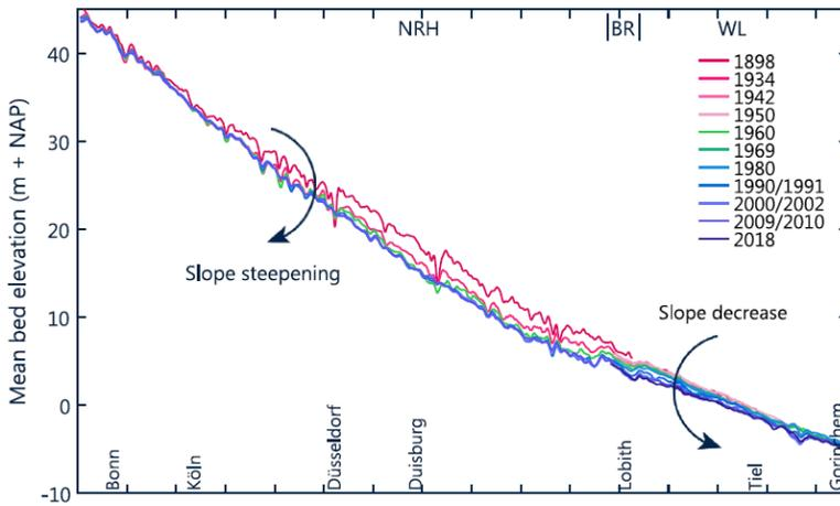
Figure 2.3: River bed erosion on the river Rhine and river Waal (Ylla Arbós et al., 2021)
