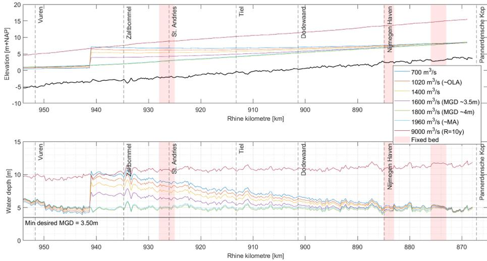
**Figure 3.8:** Upper panel: water levels for several discharges at Lobith, lower panel: water depth for several discharges
