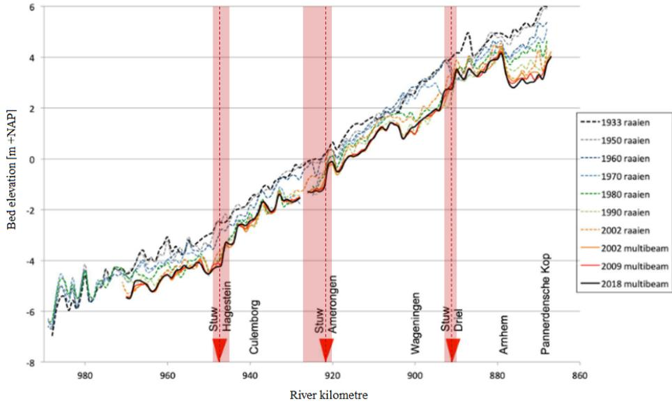
**Figure A.7:** Bed level development river Nederrijn-Lek (1933-2018). The red shaded areas indicate the deeper artificial stretches of the river that were used to construct the WLC's in (ten Brinke, 2019)
