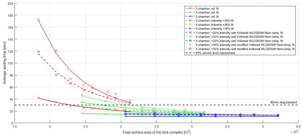
**Figure F3:** Average waiting time for all model variants for varying fleet compositions and increased traffic intensity for complex G11W5
