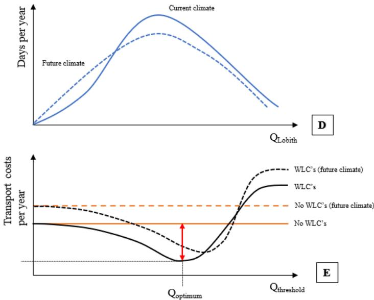
**Figure 3.2: Panel D:** conceptual discharge distributions, **Panel E:** relation between transport costs per year and discharge at Lobith (plots are based on (de Jong, 2021))
