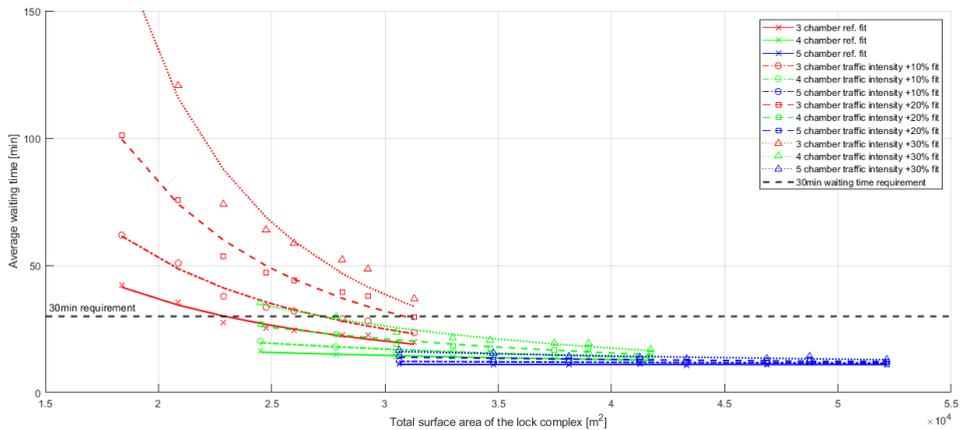
Figure E.1: Average waiting time for all model variants for varying vessel traffic intensities for complex G11W5
