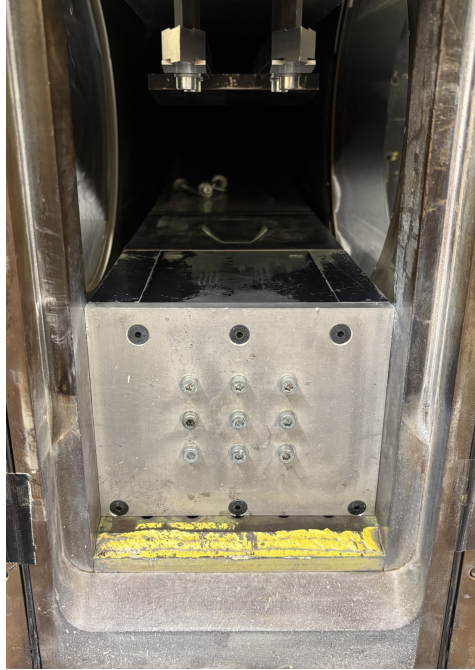
Figure 3.4: Picture of the cavity close using an aluminium plate in the ST-15 wind tunnel.
