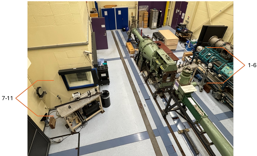
Figure 3.16: Complete Schlieren setup in the ST-15 wind tunnel including the associated numbers.
