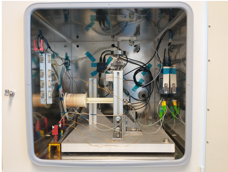
Figure 3.9: Thrust bench TB-5m inside the vacuum chamber with all sensors and equipment attached.
