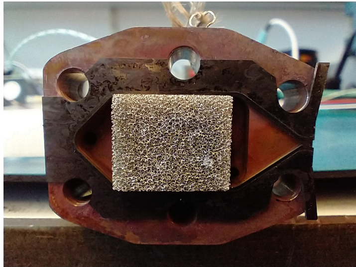
Figure 4.11: Thruster with the bottom copper block removed showing the used nozzle profile.
