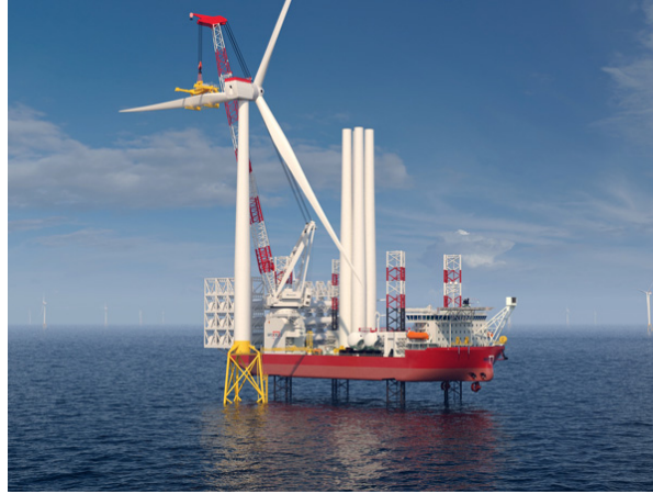
Figure 2.1: A typical jack-up used for the installation of offshore wind turbines, [18]
