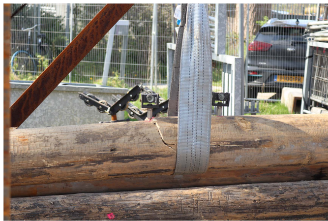
Fig. 15. Soft shell visible during loading of Pile 4 at Load step 14 of 26. The soft shell cracked open.
