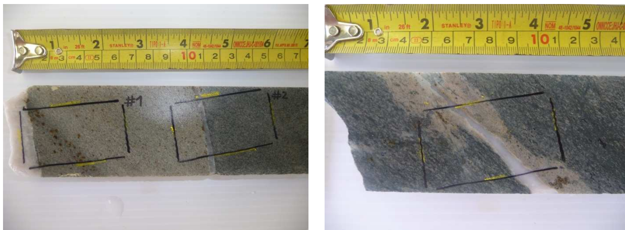
Figure 5-17, left: LC705 #1 & #2 displaying two parallel tension veins and a clear bleaching zone (KHD-603, 128.5m). Right: LC096 display of a light colour bleached zone (KHD-594, 120.8m).
