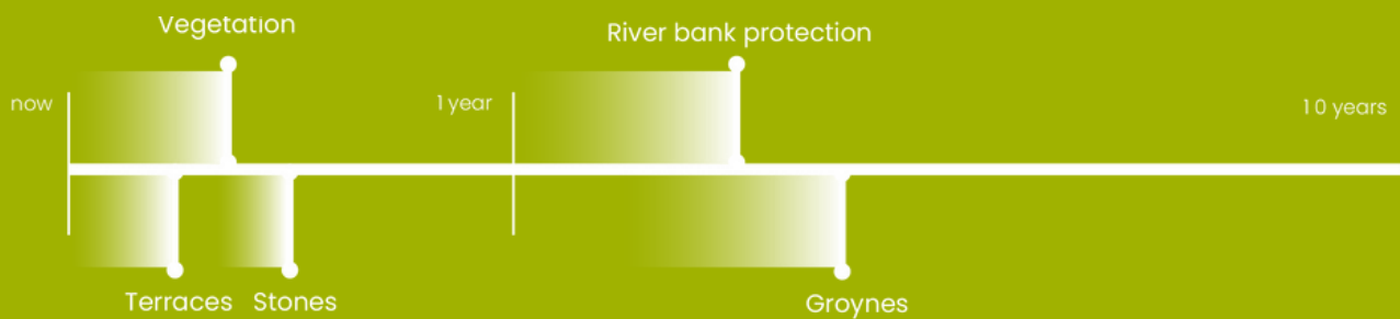
Figure 6.1: Short and long term interventions for river bank erosion (authors' work)
