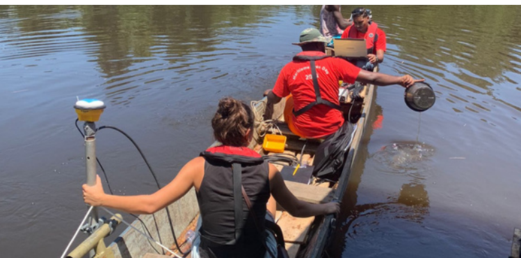
Figure 4.11: Measuring set-up for measuring wet bathymetry (authors' work)
