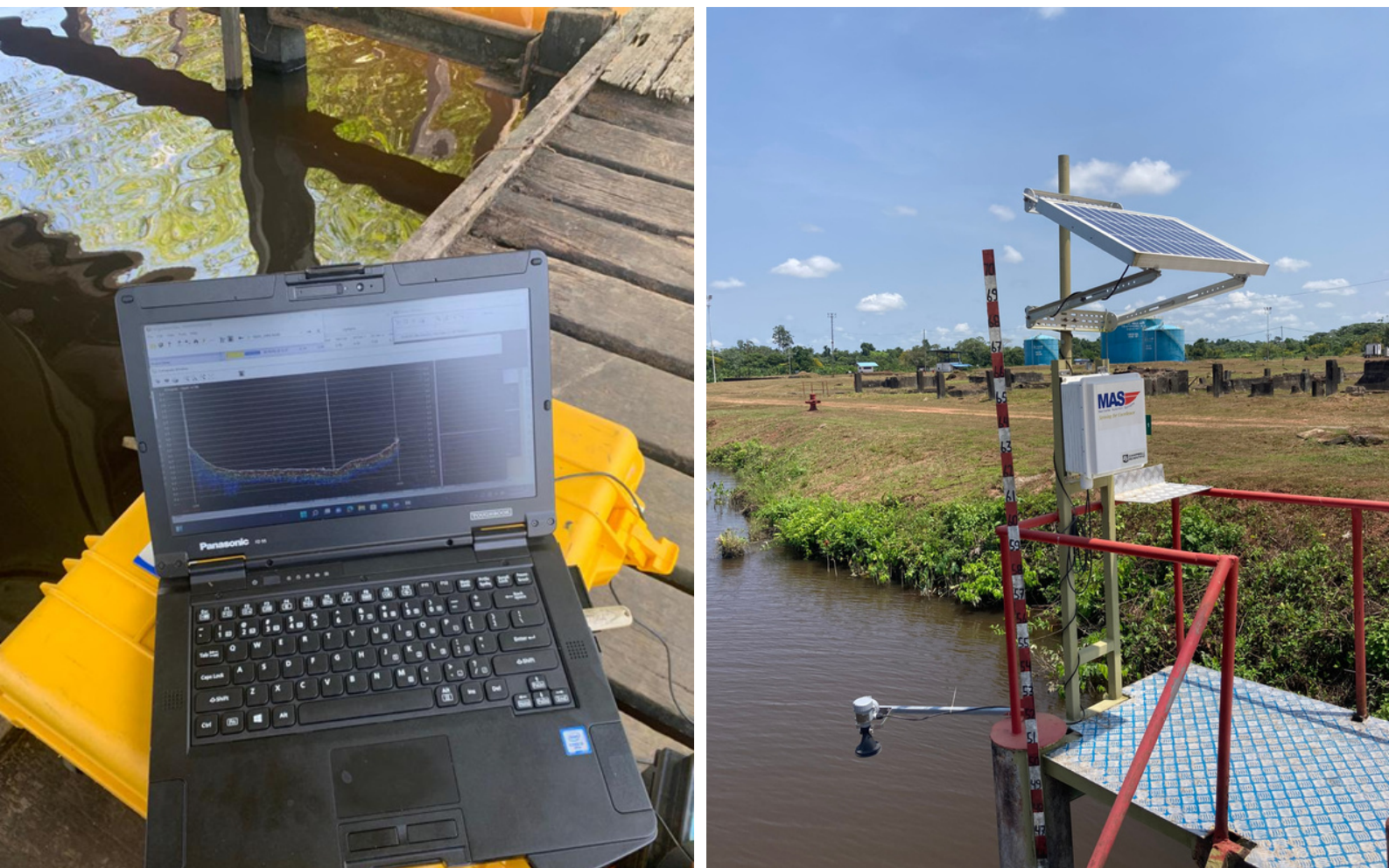
Figure 4.7: Visual representation of measurements of the bed profile (left) and water level measurements at Traymore, Moengo both by Martitieme Autoriteit Suriname
