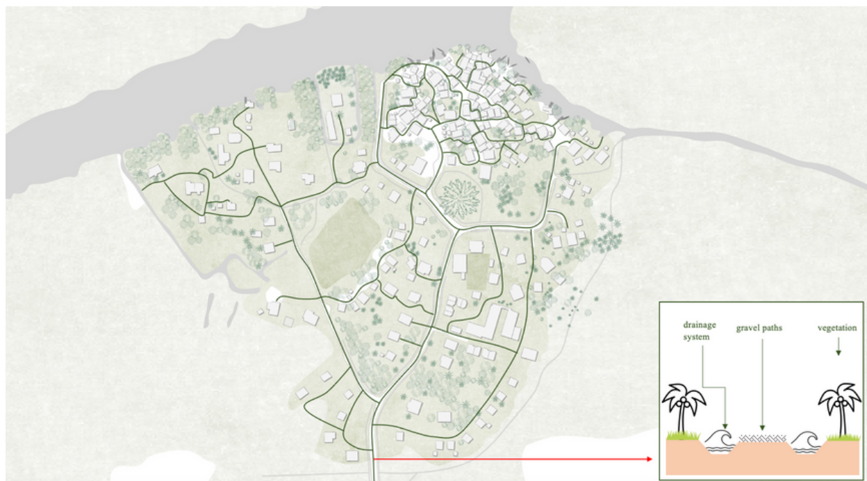
Figure 6.21: Possibilities for creating footpaths (not validated) with a small scale design of the path with vegetation and a drainage system on both sides (authors' work)
