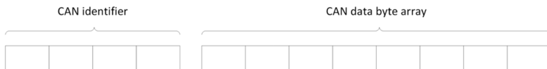
Figure 3.3: A CAN Message. Each block represents a byte.
